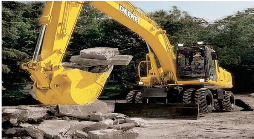
Fig. Wheeled Excavators
