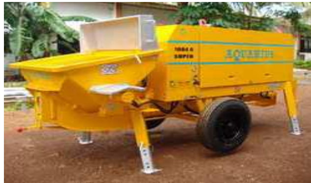
Fig. Trailer mounted concrete pump
