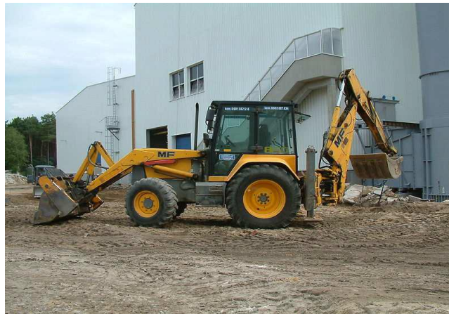
Fig. Backhoe loader
