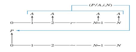
Equations 3.3 and 3.4 are each the basis for two factors tabulated in Appendix C. The series present worth factor, (P/A,i,N), and the capital recovery factor, (A/P,i,N), as shown in Equations 3.5 and 3.6, are inverses based on Equation 3.3. The capital recovery factor's name comes from asking, "How much must be saved or earned in each period, A, to recover the capital cost of the initial investment, P?"
