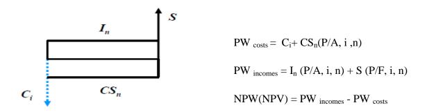
**Step 7:** In this context, a positive PW means that the equivalent worth of the inflows is greater than the equivalent worth of the outflows, so the project makes a profit. Therefore, if the PW (i) is positive for a single project, the project should be accepted; if it is negative, the project should be rejected. The process of applying the PW measure is implemented with the following decision rule:
