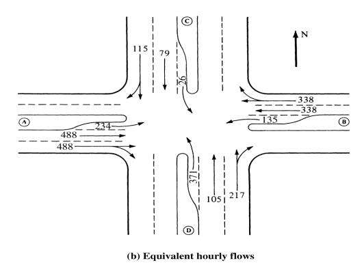
Figure 5.11a & b: Peak hour volume for major intersection on arterial highway
