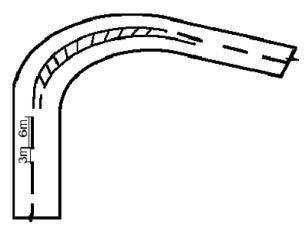
Figure 5.4: Warning line marking for a two lane road
