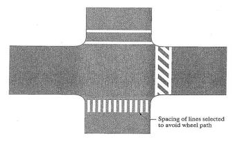
Figure 5.5: Pedestrian marking near an intersection
