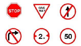
**Figure 5.7:** Examples of regulatory signs ( stop sign, give way sign, signs for no entry, sign indicating prohibition for right turn, vehicle width limit sign, speed limit sign)
