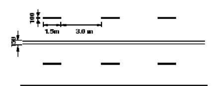
Figure 5.3: Double solid line for a two lane road
