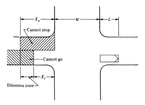
Figure 5.10 schematic of a dilemma zone.
