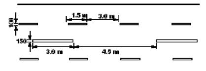
Figure 5.2: Centre line and lane marking for a four lane road
