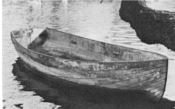
Fig. 1.1 Ferrocement Boat — “the first known example of reinforced concrete” is a boat, patented in 1848 by Joseph-Louis Lambot [Ref. : Ferrocement , National Academy of Sciences, Washington D.C., Feb. 1973]; the boat shown here is a later version (1887) of the original design, presently preserved in the Brignoles Museum, France.
