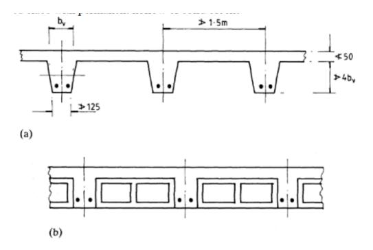
Figure 2-2 (a) Ribbed slab; (b) ribbed slab with hollow blocks
