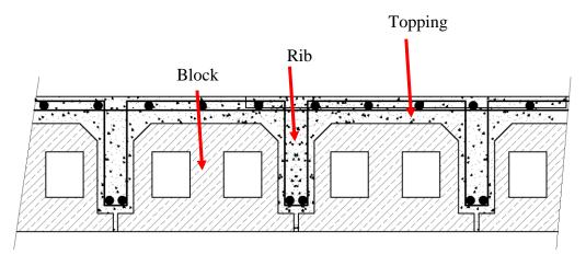
Figure 2-3 Typical ribbed slab cross-section
