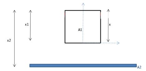
The neutral axis depth of the cracked section
