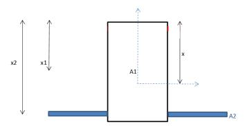
The neutral axis depth of the uncracked section
