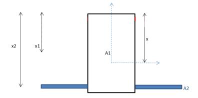
The neutral axis depth of the uncracked section
