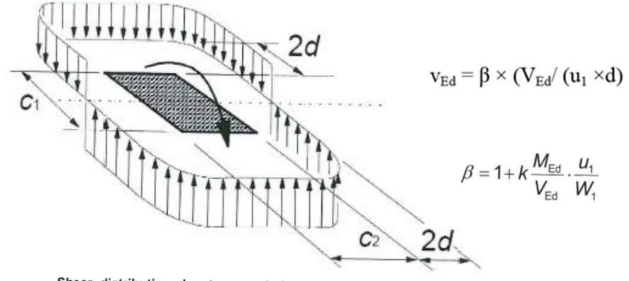
Shear distribution due to an unbalanced moment
