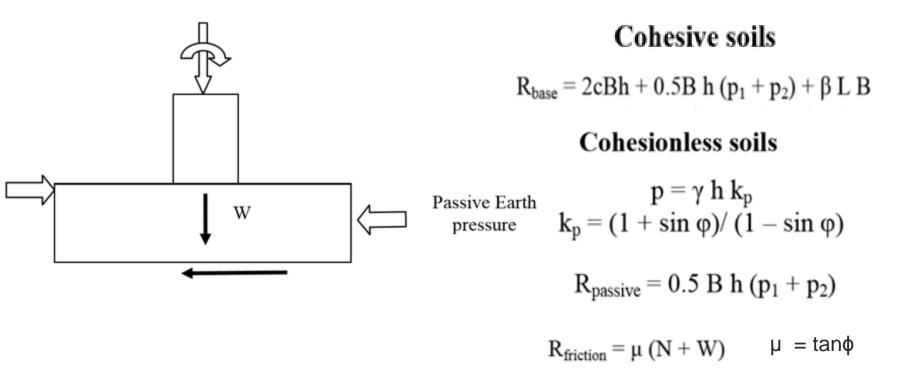
The characteristics load for an internal column footing in a building are given. The proposed dimensions for the 450 mm column square and base (3600 x 3000 mm) are shown. The base supports a ground floor slab of 200 mm thick. The soil is firm well drained clay with the following properties:
