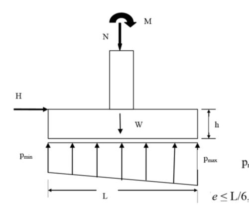
Base area  $A = B \times L$ Section modulus  $Z = B \times L^2/6$
