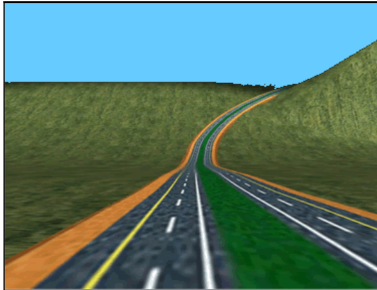
Figure I.14: Out-of-phase vertical and horizontal alignments.
