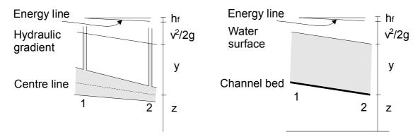
Figure of pipe and open channel flow
