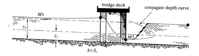
Figure of example surface profile through a bridge when in floo
