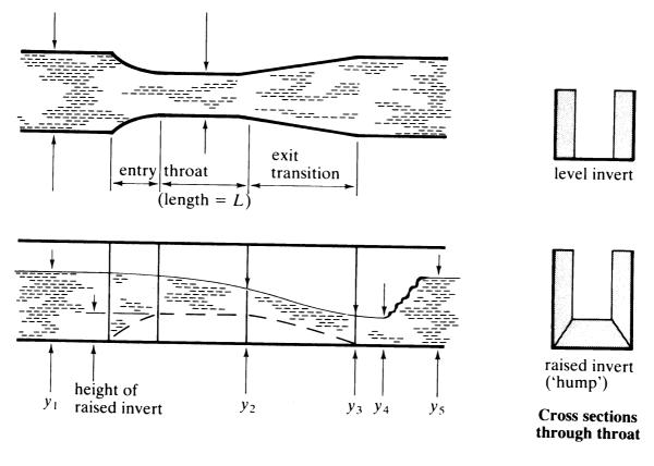
Figure of section through a Venturi flume
