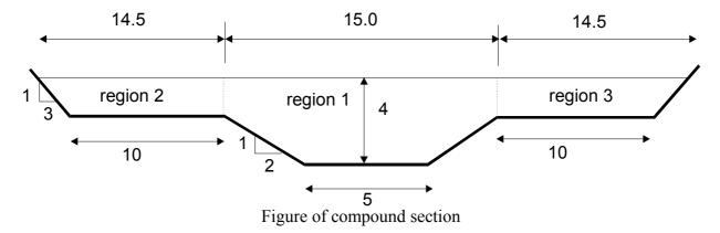
When the flow goes over the top of the trapezoidal channel it moves to the "flood plains" so the section allows for a lot more discharge to be carried.
