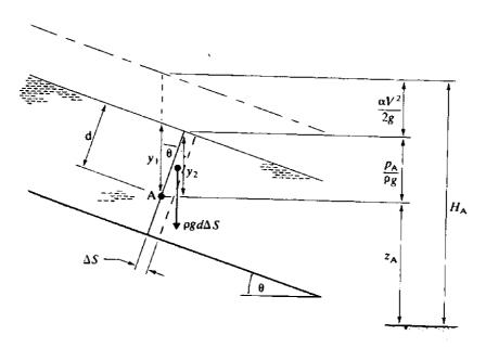
Figure of channel in uniform flow
