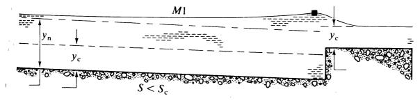
Figure of example surface profile due to a broad crested weir
