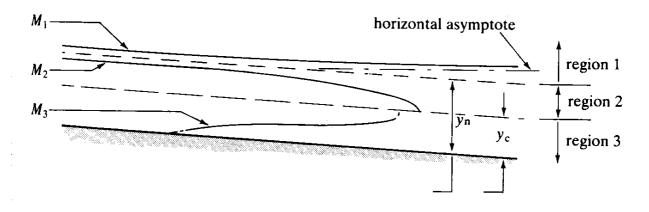
Figure of gradually varied flow surface profiles in a mild sloped channel
