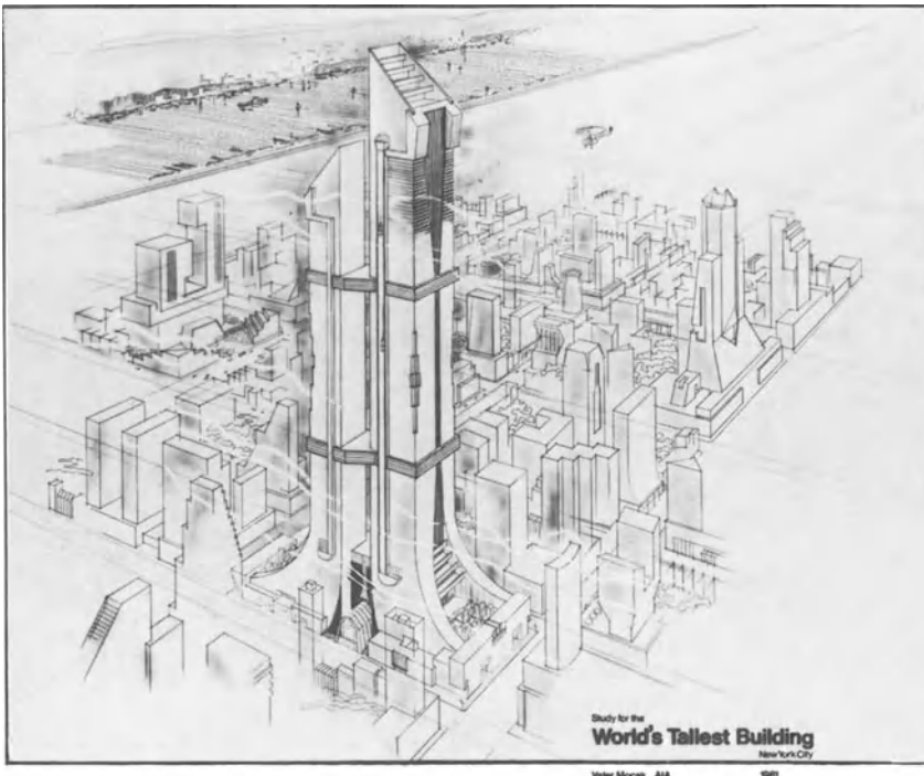
Fig. 1 Study for the “World’s Tallest Building” suggests two bridge-like skylobbies to connect two skyscrapers
