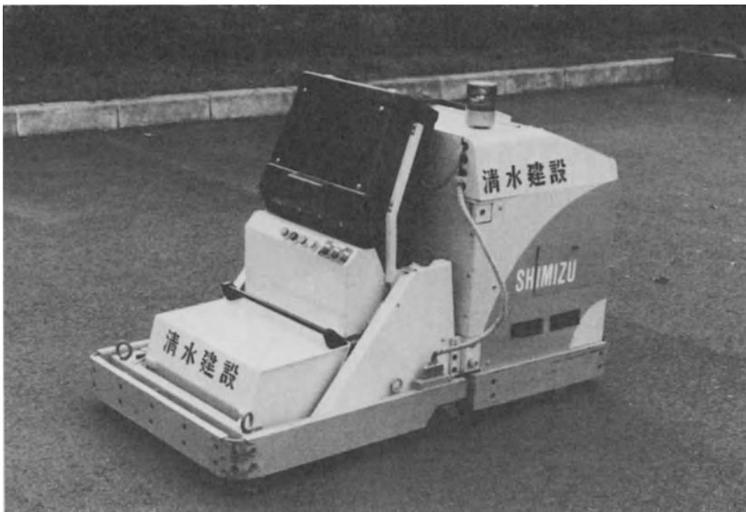
Fig. 37 Multipurpose travelling vehicle—slab surface cleaning ( Shimizu )
