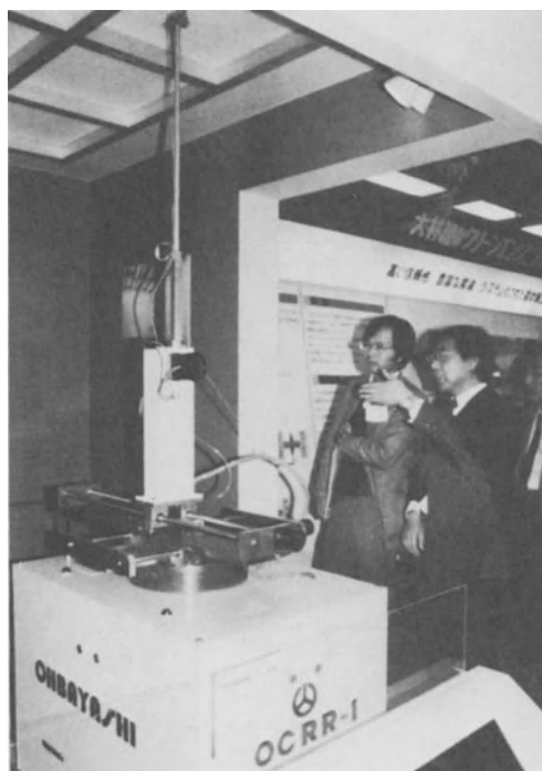
Fig. 34 Clean room testing robot ( Ohbayashi Gumi )
