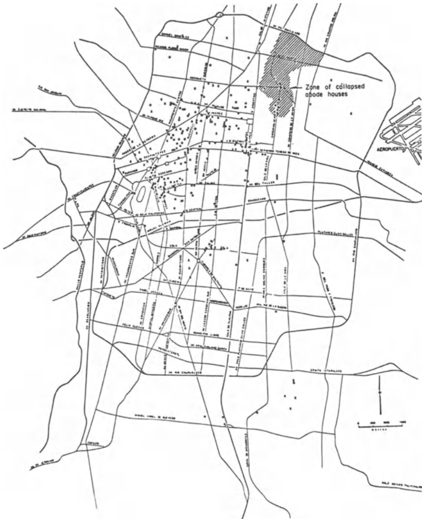
Fig. 1 Location of collapsed (●) or severely damaged (x) construction
