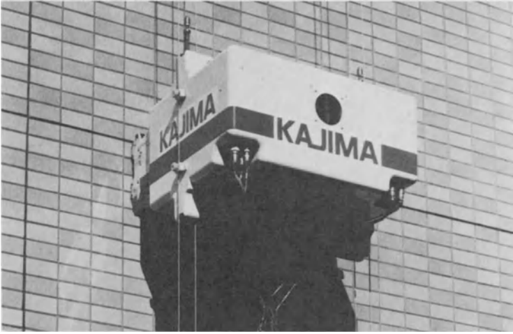
Fig. 28 Exfoliated wall tile detector ( Kajima )
