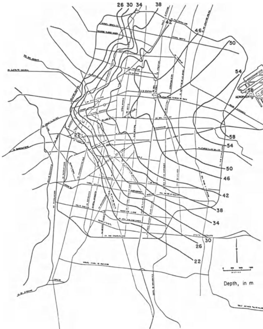
Fig. 5 Equal depth curves of the deep deposits
