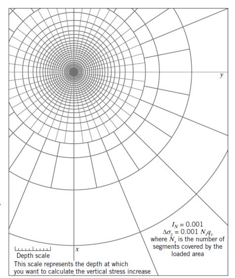
The procedure for using Newmark's chart is as follows:
