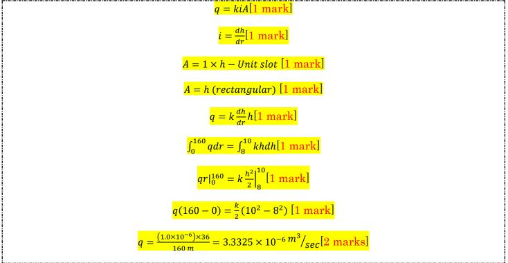
4.3 Flow of water through soils (which is analogous to steady-state heat flow and flow of current in homogeneous conductors) is described by Laplace's equation.
