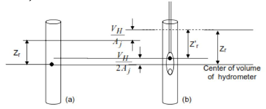
a) Before the immersion of hydrometer b) After the immersion of hydrometer
