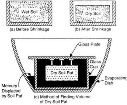
APPARATUS OF SHRINKAGE LIMIT DETERMINATION.
