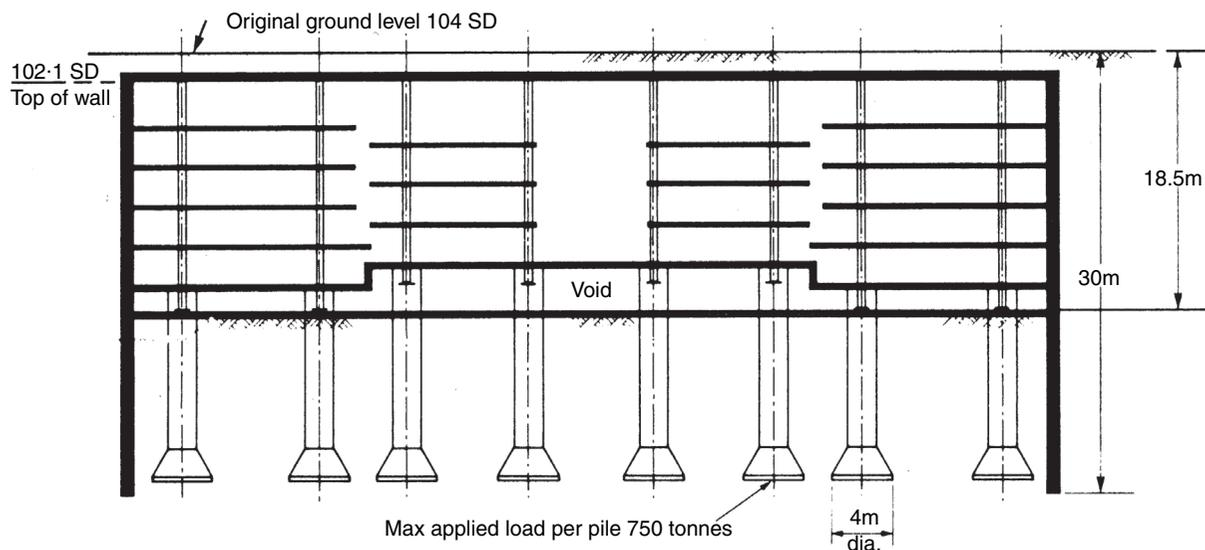
**Figure 4.3** Section through underground car park in New Palace Yard
