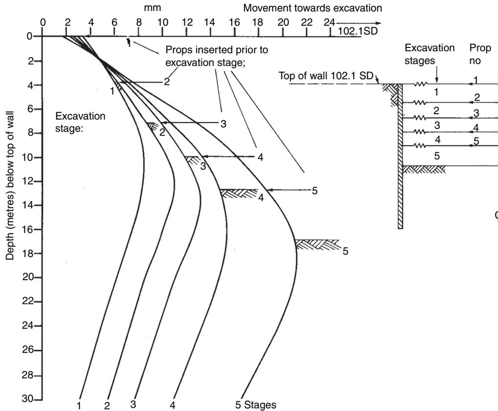
Figure 4.6 Predicted horizontal wall movements during excavation
