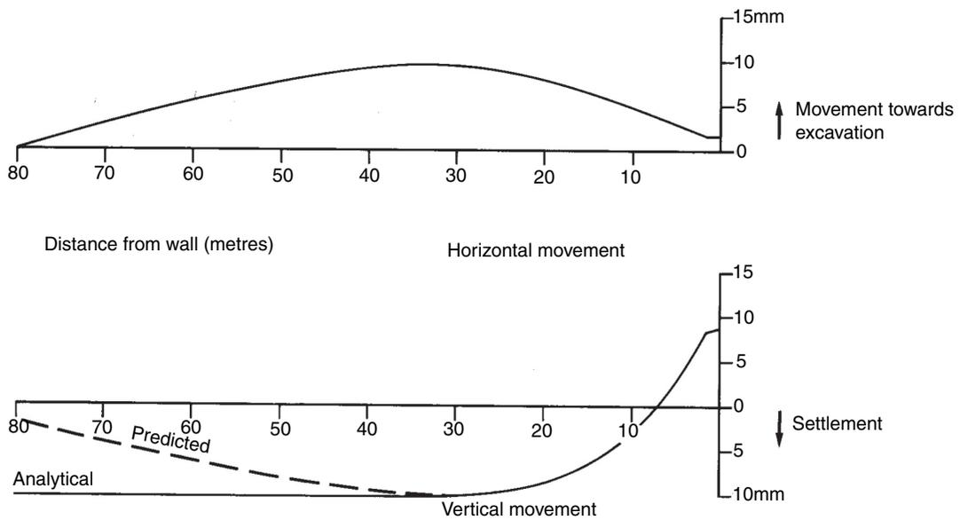
Figure 4.7 Predicted horizontal and vertical ground surface movements outside the excavation
