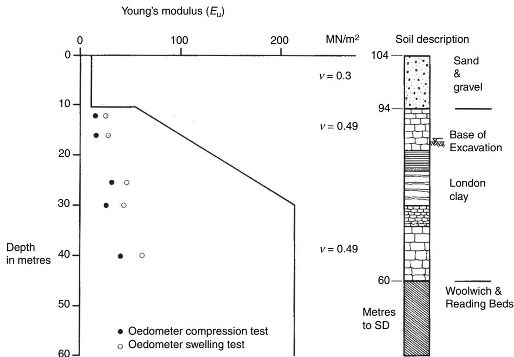
**Figure 4.5** Values of undrained Young's modulus used in the finite element analysis
