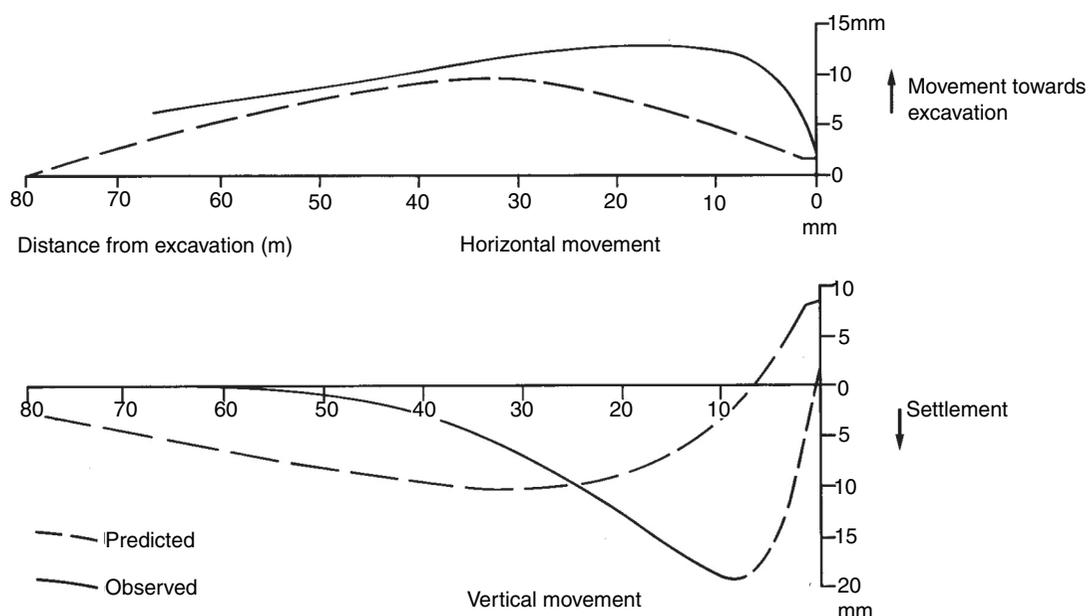
**Figure 4.9** Comparison of predicted and measured ground surface movements away from the south wall
