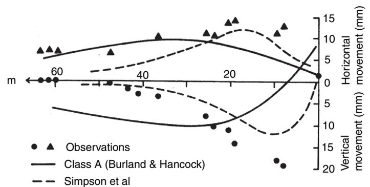
**Figure 4.10** Improved predictions of the shape of the settlement trough (shown as a broken line) due to inclusion of small strain *nonlinearity* in the soil model
