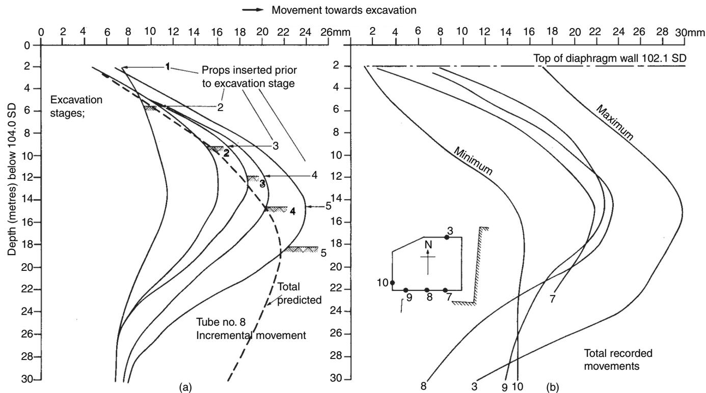
**Figure 4.8** Observed movements of the diaphragm walls. (a) Inclinometer tube 8 at various stages of excavation. (b) Range of measured movements at end of excavation
