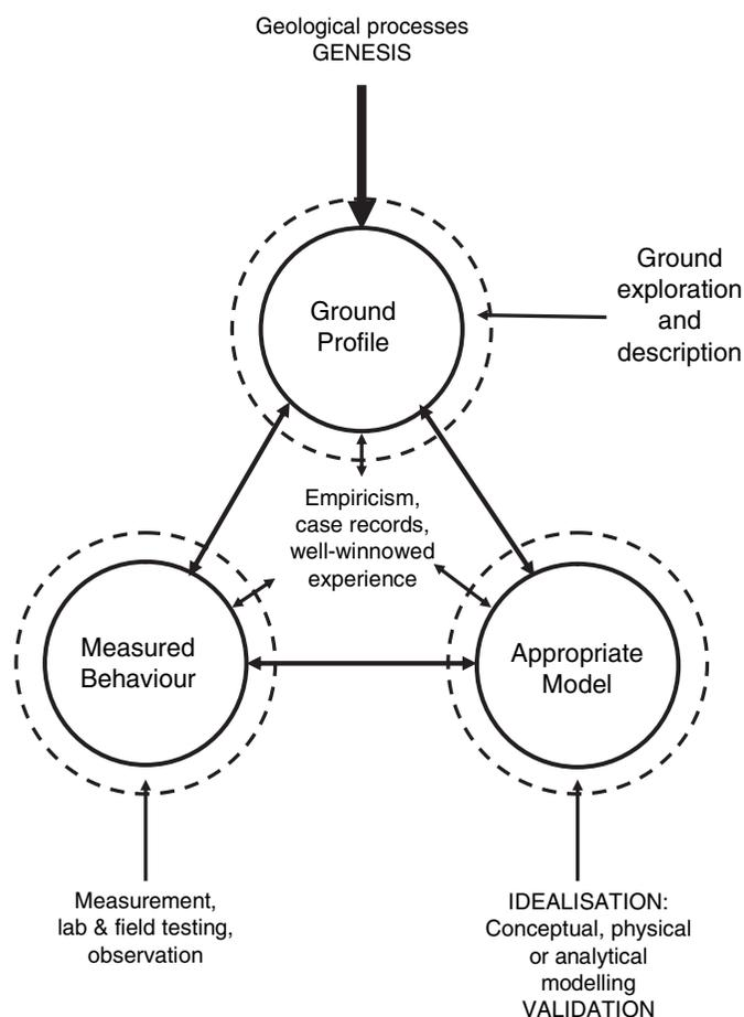
**Figure 4.1** The geotechnical triangle. Each activity has its own distinct methodology and its own rigour
