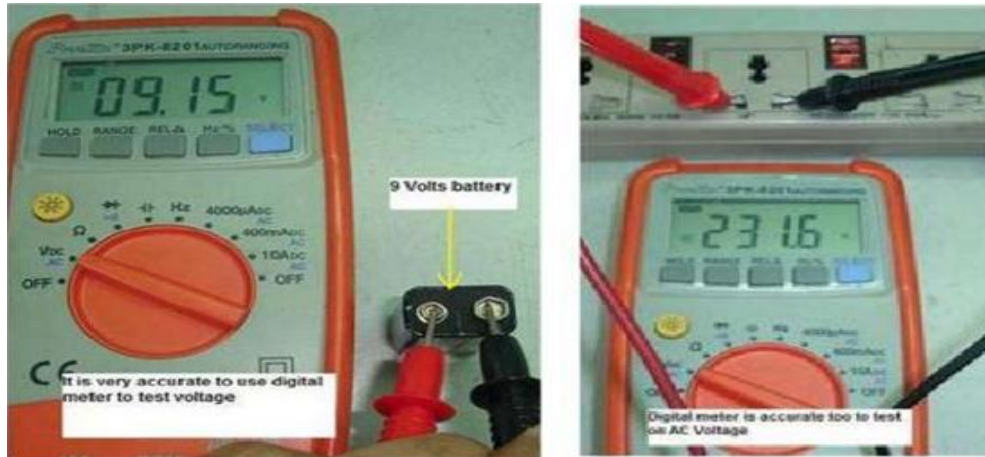
Figure6.5 Measuring the voltage using digital meter.
