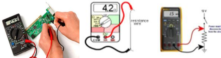
Figure6.8. Measuring the resistance (a) in the circuit (b) resistance-wire and (c)a resistor
