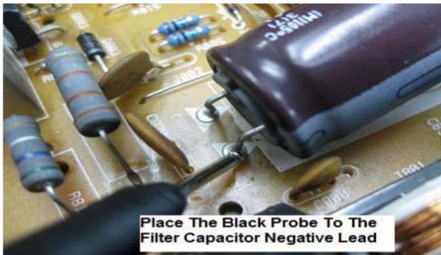
Figure3.21. Placing the BLACK test probe to the negative pin of the Filter Capacitor.
