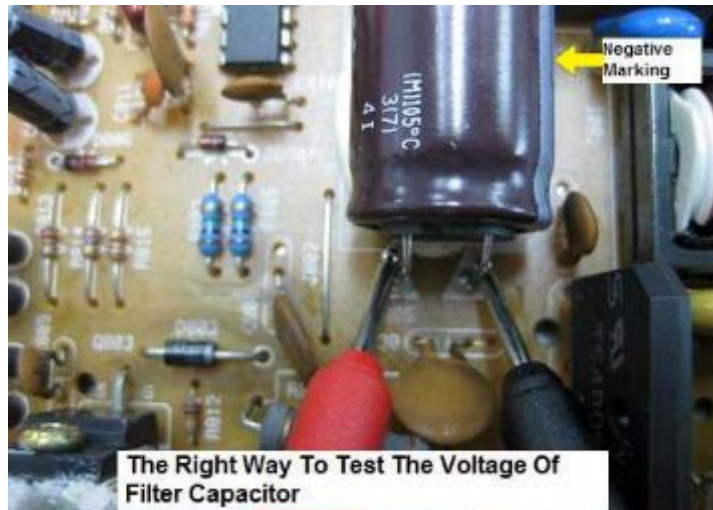
Figure3.19. Testing voltage at the filter capacitor
