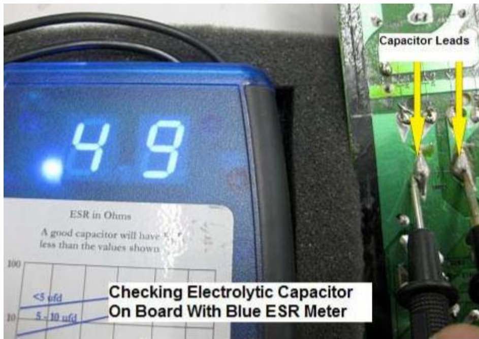
Figure5.6. Checking the electrolytic capacitor using Blue ESR meter
