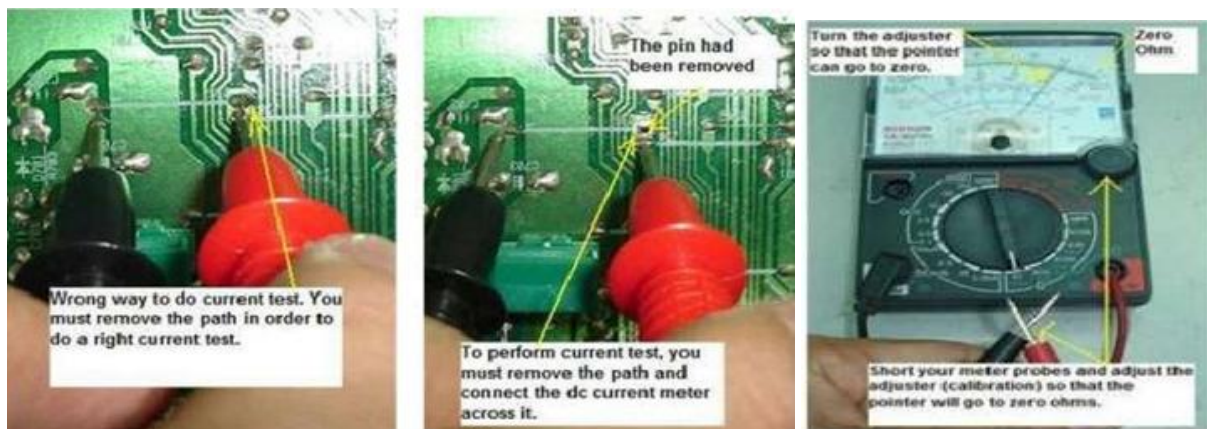
Figure6.5 Measuring current in a circuit
