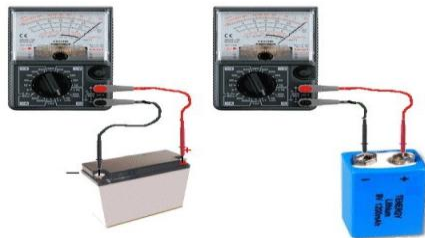
Figure6.9. Caution in measuring resistance
