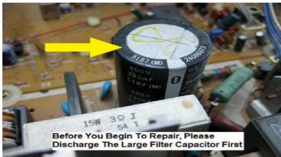
Figure5.2 Discharging the Big Capacitor with a 2.2Kohm 10watt resistor
