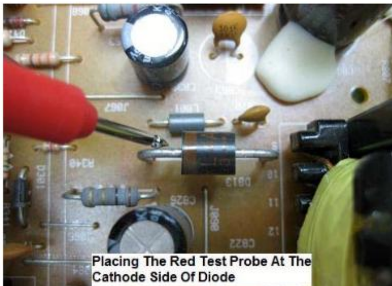
Figure3.23. Placing the RED test probe to the Secondary Output Diode Cathode Side.
