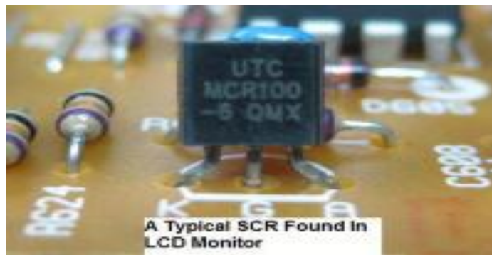
Figure4.93. Silcom Controlled Rectifier
