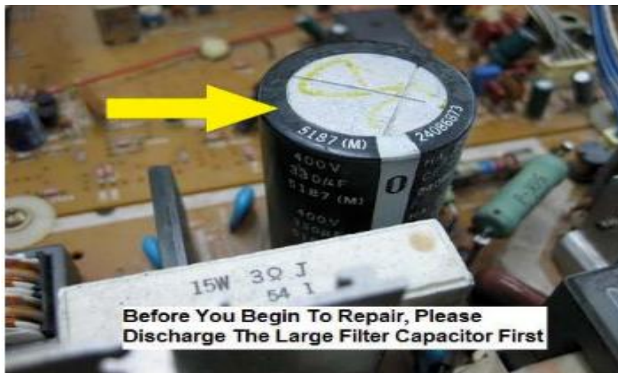
Figure5.1 Discharging the Big Capacitor
