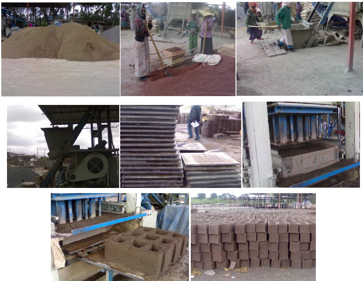
Fig. 5.3.37 Manufacturing of concrete masonry blocks
