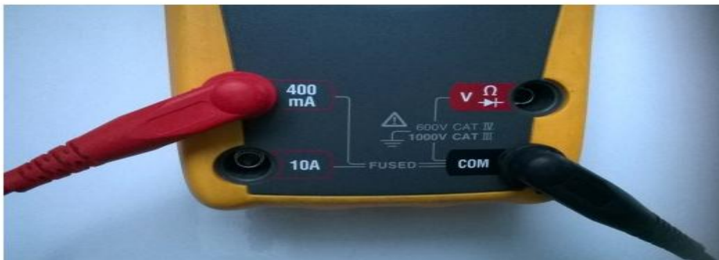
Test leads and sockets on a DMM, setup to measure current | Source
