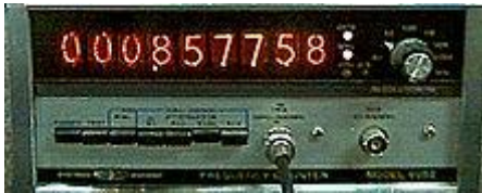
Systron-Donner frequency counter from 1973 with Nixie tube display
