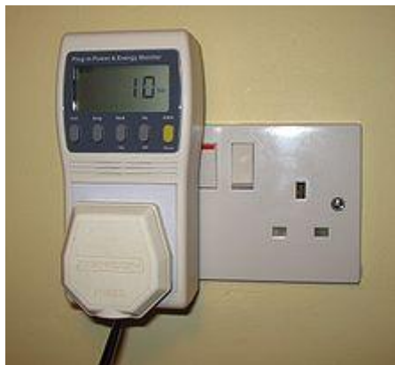
Prodigit Model 2000MU (UK version), shown in use and displaying a reading of 10 watts being consumed by the appliance
