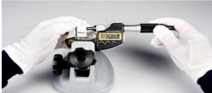
Fig. 2.62. After using steel gauge blocks, clean and apply rust prevention treatment
