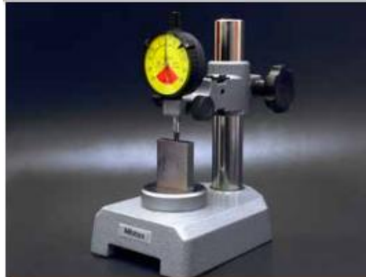
Fig.2.57. Reference point setting with a 50 mm Gauge Block.
