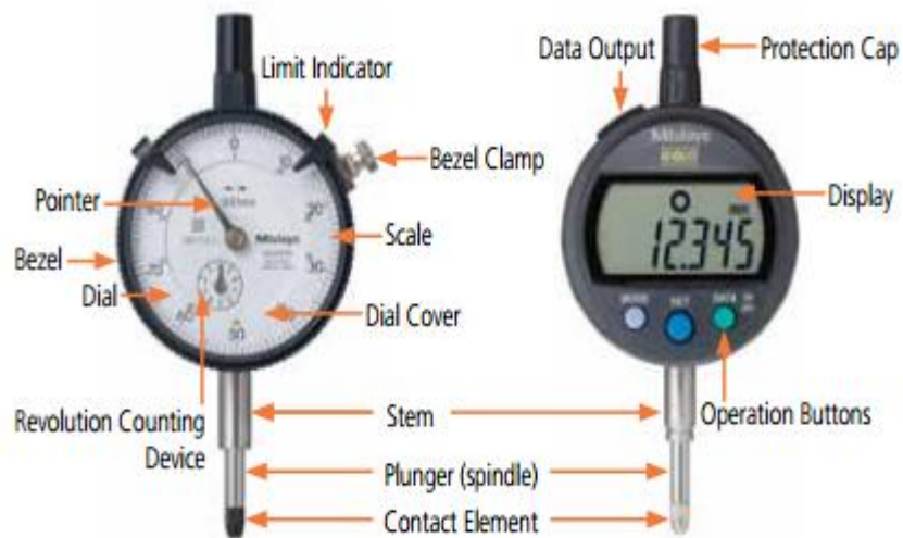
Fig.2.44. parts of indicator
