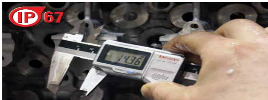
Fig. 2.16. to check the dimension of gear
