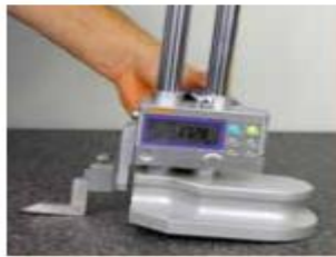
Excessive downwards force lifting the base from the plate
