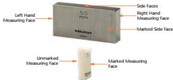
Fig. 2.59. parts of gauge block Before Use
