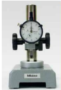
fig.2.5. Zero setting with a 10 mm ceramic gauge block if the work piece nominal is 10 mm
