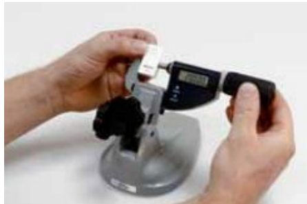
Fig.2.4. Reference point setting with a gauge block
