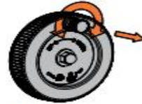
Fine feed To use fine feed, pull the handle out and rotate its sleeve.
