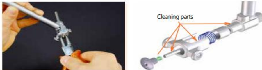
Fig.2.34. film of micrometer oil to the contact point and the driver pin.
