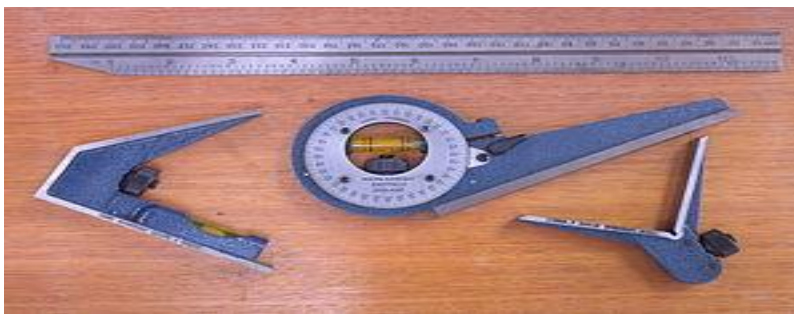
Fig. 1.7. combination square Uses
