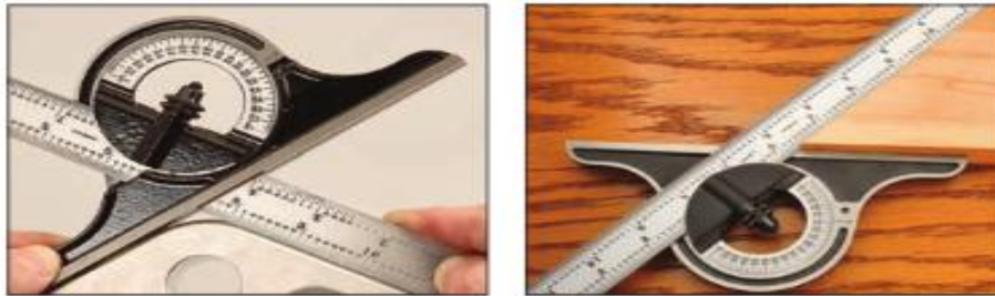
Fig. 3.14. Application a combination square.
