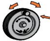
Coarse feed To use coarse feed push the handle in and rotate the whole wheel.
