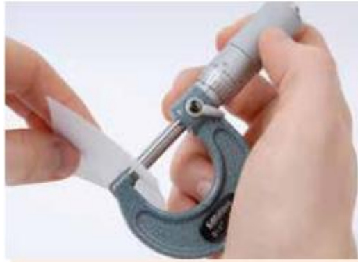
Fig. 2.20. how to use micro meter
