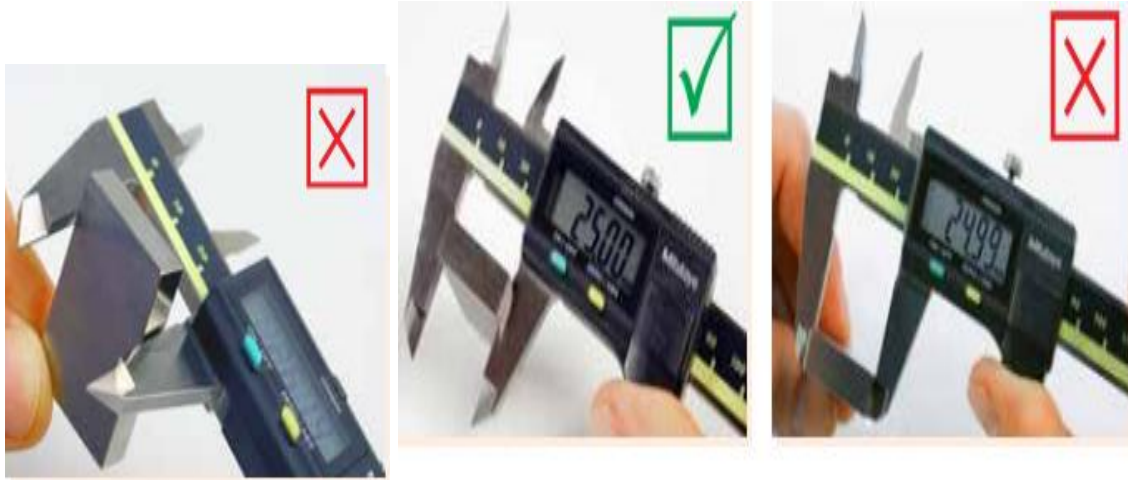
Fig.2.37. correct use of calipers
