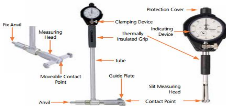
Fig.2.29. 2. parts of -Point Internal Measuring Instruments
