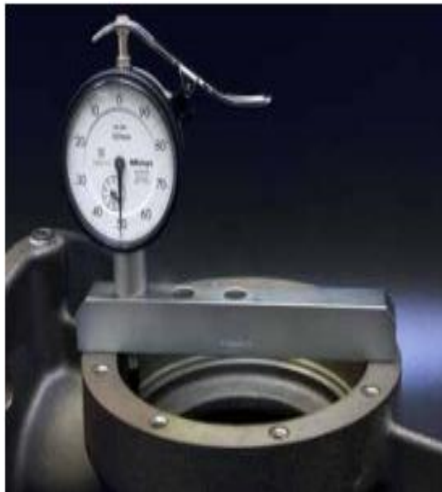
Fig. 2.55. use the gauge in vertical orientation only.
