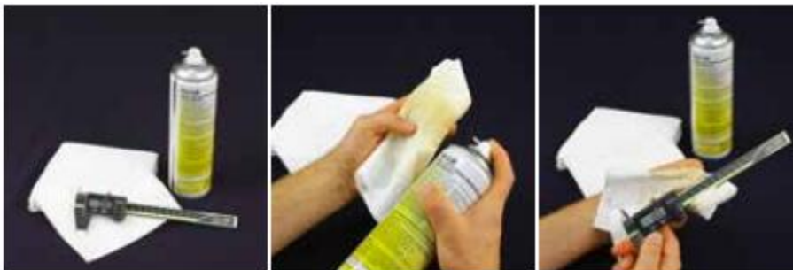
Fig.2.10. apply anti-corrosive coating for rust prevention
