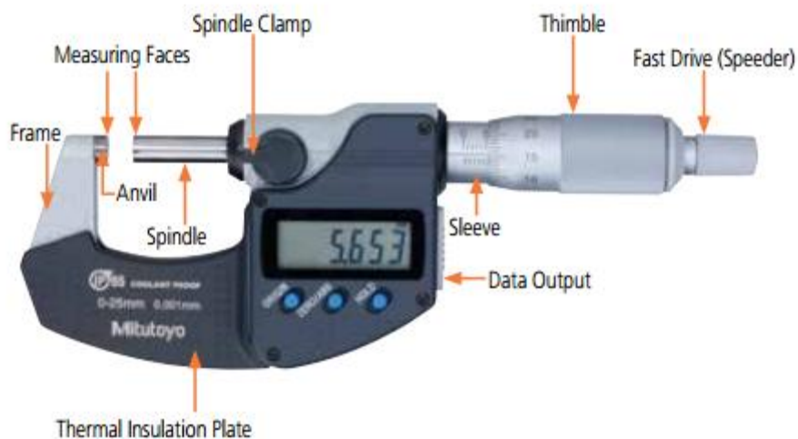
Fig. 2.19. parts of out side micro meter
