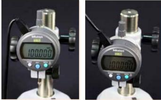
Fig.2.17. Avoid abnormal cable guidance and tensile stress
