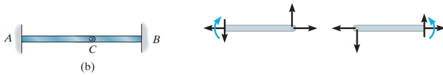
The compound beam is *stable*. It is also indeterminate to the second degree. *Ans.*
