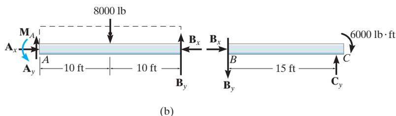
**Equations of Equilibrium.** There are six unknowns. Applying the six equations of equilibrium, using previously calculated results, we have
