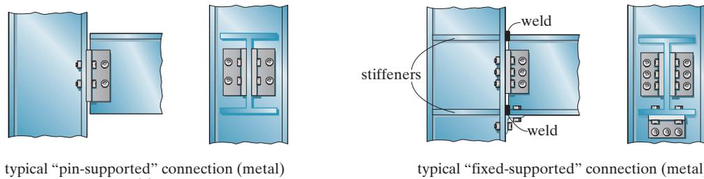
**Idealized Structures**—By making assumptions about the supports and connections as being either hinged, pinned, or fixed, the members can then be represented as lines, so that we can establish an idealized model that can be used for analysis.
