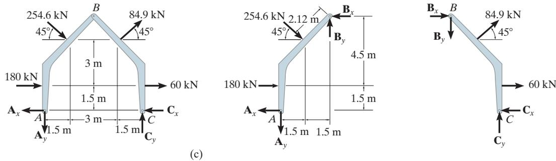
**Equations of Equilibrium.** Simultaneous solution of equations is avoided by applying the equilibrium equations in the following sequence using previously computed results.\*
