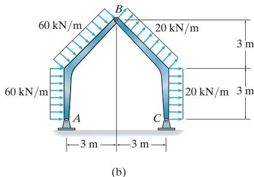
**Free-Body Diagrams.** Simplifying the distributed loadings, the free-body diagrams of the entire frame and each of its parts are shown in Fig. 2-33c.
