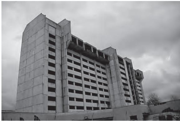
The “shear walls” on the sides of this building are used to strengthen the structure when it is subjected to large hurricane wind loadings applied to the front or back of the building.
