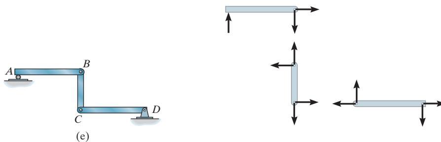
The structure is *unstable* since  $r = 7$ ,  $n = 3$ , so that, by Eq. 2-4,  $r < 3n$ ,  $7 < 9$ . Also, this can be seen by inspection, since *AB* can move horizontally without restraint. *Ans.*
