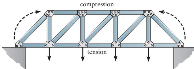
Loading causes bending of truss, which develops compression in top members, tension in bottom members
