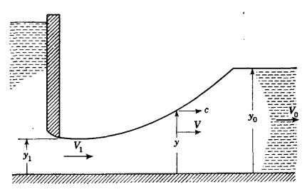
Fig. 11.19. Negative wave after gate closure.
