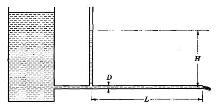
Fig. 9.39. Determination of viscosity by flow through a capillary tube.
