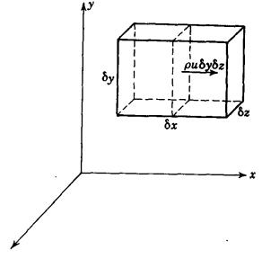
$$\left[\frac{\partial}{\partial x}(\rho u) + \frac{\partial}{\partial y}(\rho v) + \frac{\partial}{\partial z}(\rho w)\right] \delta x \, \delta y \, \delta z \quad \text{Fig. 3.6. Time rate of mass flow through a face.}$$
