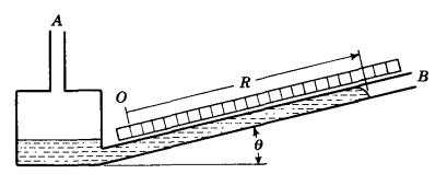
Fig. 2.13. Inclined manometer.
