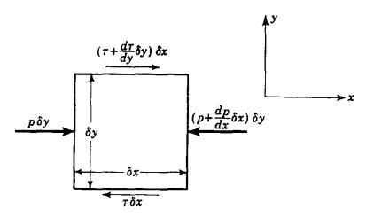
Fig. 5.3. Forces on a fluid element.
