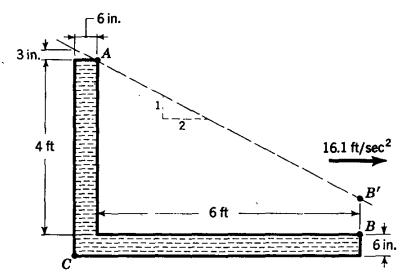
Fig. 2.15. Tank completely filled with liquid.
