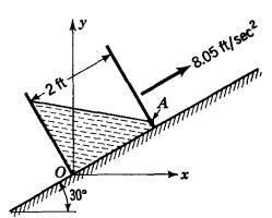
Fig. 2.17. Uniform acceleration along an inclined plane.
