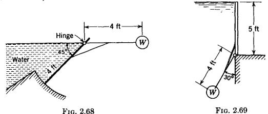
2.93. The gate of Fig. 2.69 weighs 100 lb/ft normal to the page. It is in equilibrium as shown. Neglecting the weight of the arm and brace supporting the counterweight, (a) determine W and (b) determine whether the gate is in stable equilibrium. The weight is made of concrete, sp gr 2.50.
