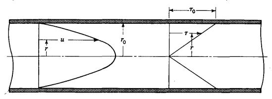
Fig. 5.7. Velocity distribution and shear-stress distribution in laminar flow in a round tube.
