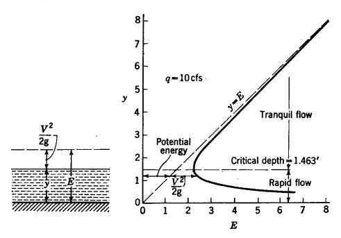
Fig. 11.7. Specific energy required for flow of a given discharge at various depths.
