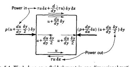
Fig. 5.4. Work done on a fluid element in one-dimensional motion.
