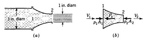
Fig. 3.20. Nozzle at the end of a pipe.
