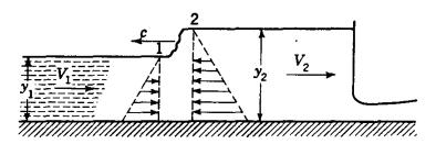
Fig. 11.16. Positive surge wave in a rectangular channel.
