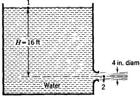
Fig. 3.12. Flow from a reservoir.
