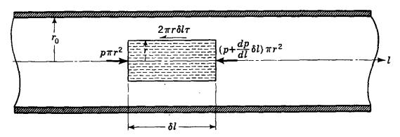
Fig. 5.6. Free-body diagram for steady flow through a round tube.
