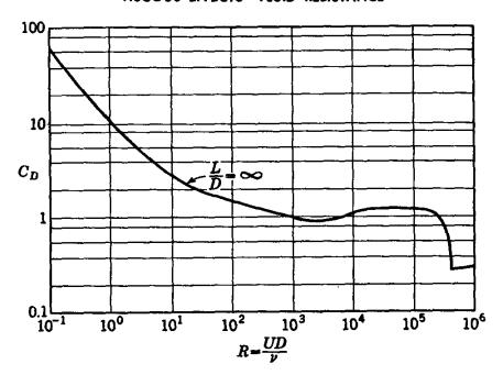
Fig. 5.24. Drag coefficients for circular cylinders.
