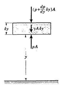
Fig. 2.4. Free-body diagram for vertical forces acting on a fluid element.
