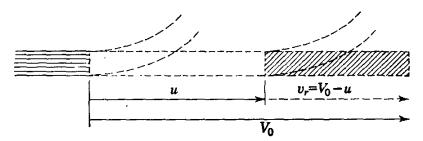
Fig. 3.29. Fluid overtaking vane in 1-sec period.
