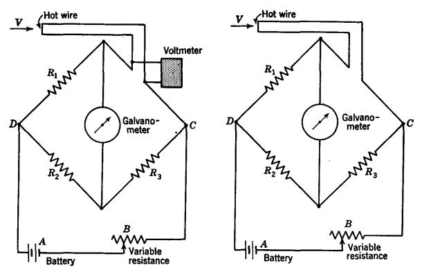
Fig. 9.8. Constant-resistance hot-wire anemometer.
