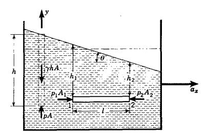
Fig. 2.14. Horizontal acceleration.
