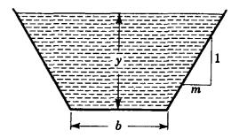
Fig. 5.29. Notation for trapezoidal cross section.
