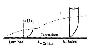
Fig. 5.18. Boundary-layer growth. (The vertical scale is greatly enlarged.)
