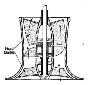
Fig. 8.21. Axial-flow pump. (Ingersoll-Rand Co.)
