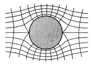
Fig. 7.30. Equipotential lines and streamlines for flow around a circular cylinder.
