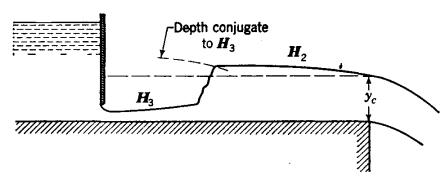
Fig. 11.13. Hydraulic jump between two control sections.
