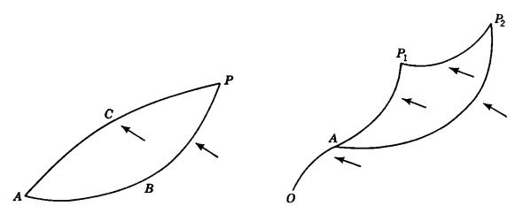
Fig. 7.7. Fluid region showing the positive flow direction used in the definition of a stream function.
