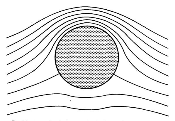
Fig. 7.31. Streamlines for flow around a circular cylinder with circulation.
