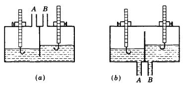
Fig. 2.11. Hook-gage micromanometers. (a) For gases; (b) for liquids.
