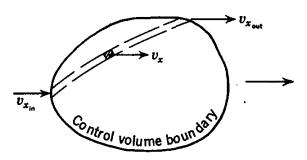
Fig. 3.17. Control volume for derivation of momentum equation.
