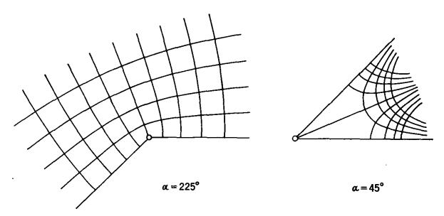
Fig. 7.25. Flow net for flow along two inclined surfaces.
