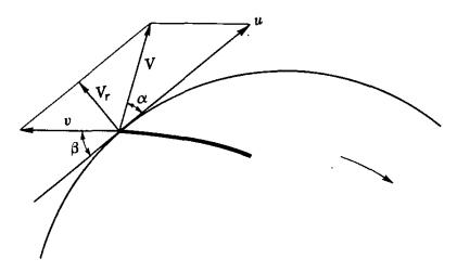
Fig. 8.1. Velocity vector diagram for exit from a pump impeller.
