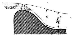
Fig. 11.6. Example of specific energy.
