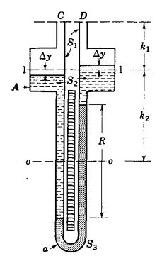
Fig. 2.12. Micromanometer using two gage liquids.
