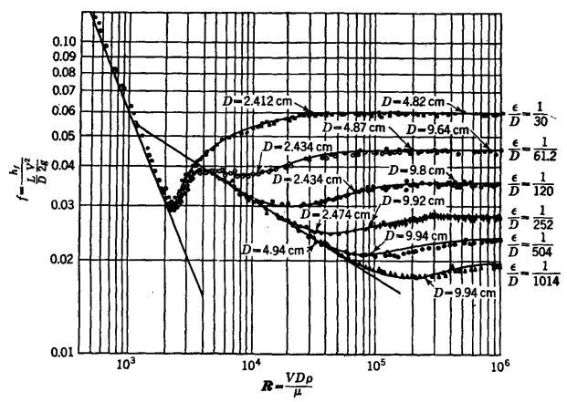
Fig. 5.33. Nikuradse's sand-roughened-pipe tests.
