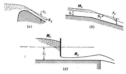
Fig. 11.12. Channel control sections.
