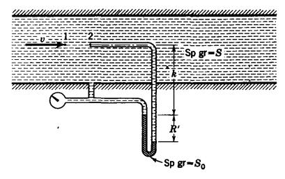
Fig. 9 6. Use of pitot tube and piezometer opening for measurement of velocity.
