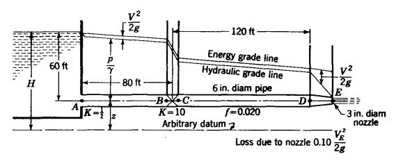
Fig. 10.1. Hydraulic and energy grade lines.
