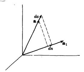
Fig. 7.5. Change of vector a corresponding to change in normal direction.
