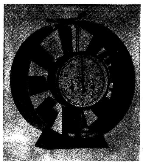
Fig. 9.11. Air anemometer. (Taylor Instrument Co.)
