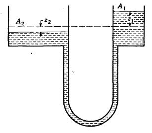
Fig. 10.16. Oscillation of two reservoirs.
