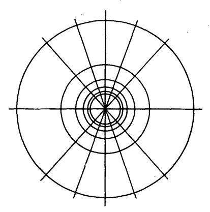
Fig. 7.16. Streamlines and equipotential lines for a source.
