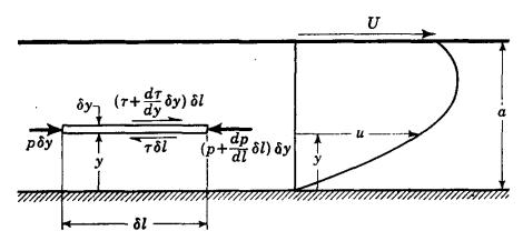
Fig. 5.1. Flow between parallel plates with upper plate in motion.
