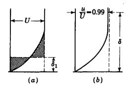
Fig. 5.16. Definitions of boundary-layer thickness.
