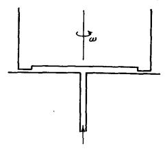
Fig. 5.40. Hydrostatic lubrication by high-pressure pumping of oil.
