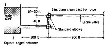
Fig. 5.37. Pipeline with minor losses.
