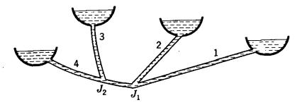
Fig. 10.9. Four reservoirs with two junctions.
