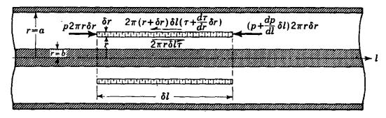
Fig. 5.11. Free-body diagram for flow through an annulus.
