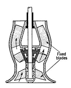
Fig. 8.22. Mixed-flow pump. (Ingersoll-Rand Co.)
