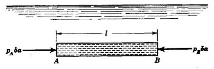
Fig. 2.2. Two points at same elevation in a static fluid.
