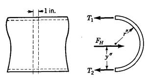
Fig. 2.32. Tensile stress in pipe.
