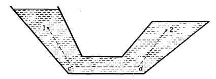
Fig. 2.3. Paths for considering variation of pressure in a fluid.
