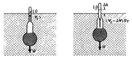
Fig. 2.36. Hydrometer, in water and in liquid of specific gravity S.
