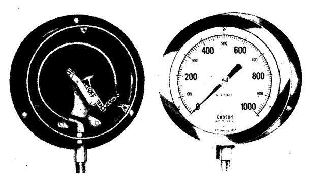
Fig. 2.5. Bourdon gage. (Crosby Steam Gage and Valve Co.)
