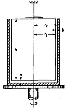
Fig. 9.37. Concentric-cylinder viscometer.
