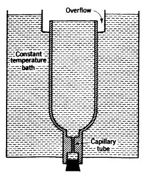
Fig. 9.40. Schematic view of Saybolt viscometer.
