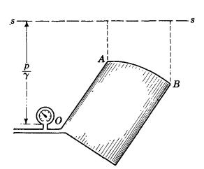
Fig. 2.29. Vertical component of force on a curved surface.
