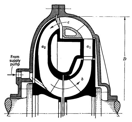
Fig. 8.34. Torque converter with two-stage turbine.  $(a_1)$  First-stage turbine;  $(a_2)$  second-stage turbine; (b) pump; (c) stationary guide vanes; (d) maximum diameter of circuit. (David Taylor Model Basin, U.S. Navy Dept.)
