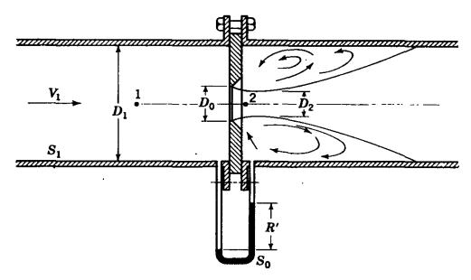
Fig. 9.27. Orifice in a pipe.
