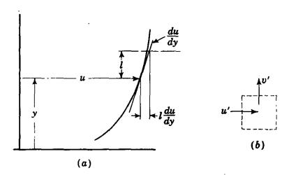
Fig. 5.14. Notation for mixing-length theory.
