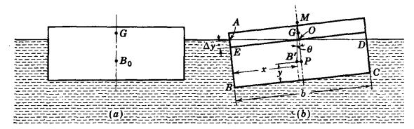
Fig. 2.39. Stability of prismatic body.
