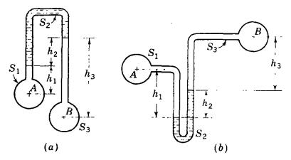
Fig. 2.9. Differential manometers.
