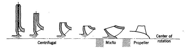
Fig. 8.25. Impeller types used in pumps and blowers. (Worthington Pump and Machinery Corp.)
