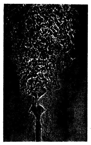
Fig. 9.15. Shadowgraph view of propaneair combustion. Flame is stabilized around  $\frac{1}{16}$ -in.-diameter spherical flame holder at bottom. Jet velocity 77 ft/sec. (Willow Run Research Center, The University of Michigan.)
