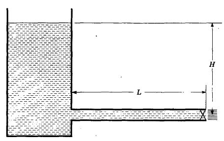
Fig. 10.17. Notation for establishment of flow.
