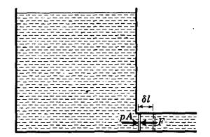
Fig. 3.9. Work done by sustained pressure force.
