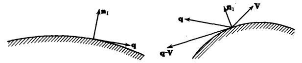
Fig. 7.11. Notation for boundary condition at a fixed boundary.
