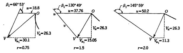
Fig. 8.19. Velocity diagrams for angle of leading edge of a propeller turbine blade.
