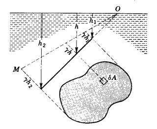
Fig. 2.24. Illustration of pressure prism.
