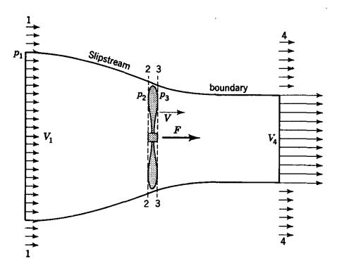
Fig. 3.21. Propeller in a fluid stream.
