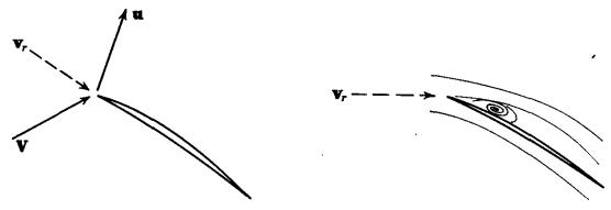
Fig. 8.5. Relative velocity tangent to blade.
