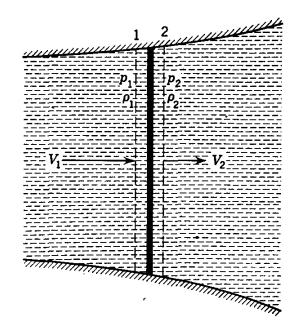
Fig. 6.2. Normal compression shock wave.
