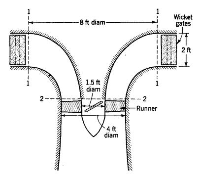
Fig. 8.9. Schematic view of propeller turbine.
