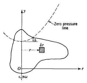
Fig. 2.18. Rotation of fluid about a vertical axis.
