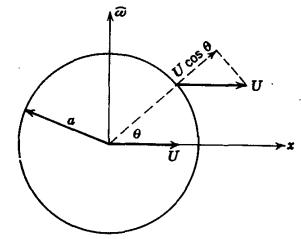
Fig. 7.21. Sphere translating in the positive x-direction.
