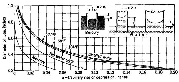
Fig. 1.4. Capillarity in circular glass tubes. (By permission from "Hydraulics," by R. L. Daugherty, copyright 1944, McGraw-Hill Book Company, Inc.)
