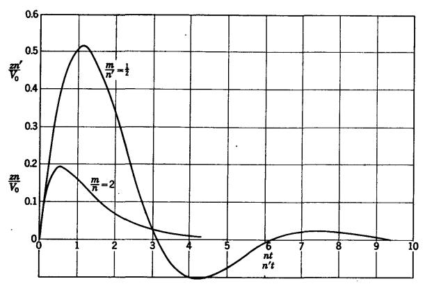
Fig. 10.14. Position of meniscus as a function of time for oscillation of liquid in a U-tube with laminar resistance.
