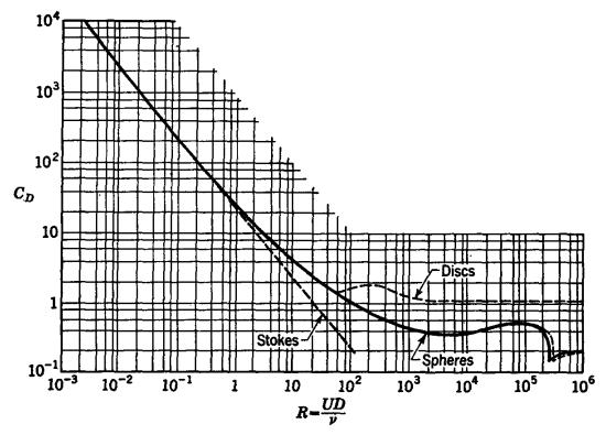
Fig. 5.23. Drag coefficients for spheres and circular disks.
