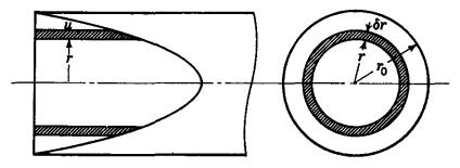
Fig. 5.8. Ring element of area used to compute discharge.
