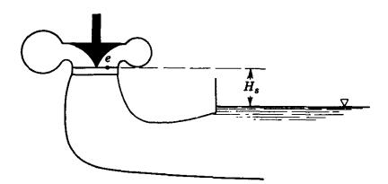
Fig. 8.36. Turbine or pump setting.
