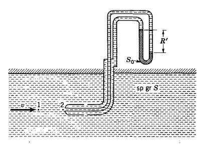
Fig. 9.7. Pitot-static tube.
