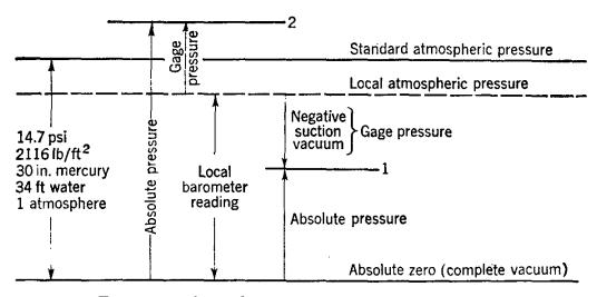
Fig. 2.6. Units and scales for pressure measurement.
