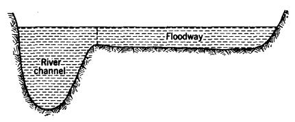
Fig. 11.3. Floodway cross section.
