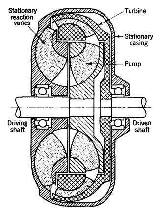
Fig. 8.33. Torque converter
