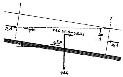
Fig. 5.28. Axial forces on free body of fluid in a conduit.
