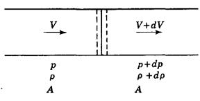
Fig. 6.1. Steady flow in prismatic channel with sudden small change in velocity, pressure, and density.
