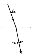
Fig. 9.12. Angles of incidence and refraction.
