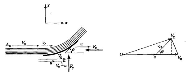
Fig. 3.28. Velocity relationships for a moving vane.
