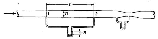
Fig. 5.32. Experimental arrangement for determination of head loss in a pipe.
