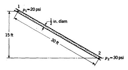
Fig. 5.10. Flow through an inclined tube.
