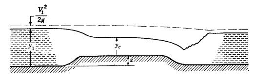
Fig. 11.15. Critical-depth meter.
