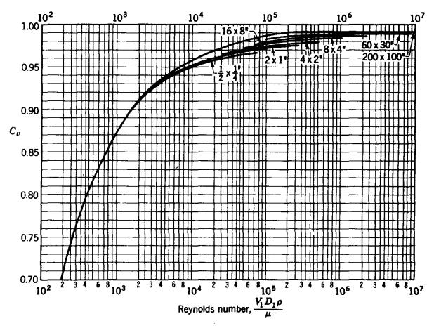
Fig. 9.24. Coefficient C, for venturi meters ("Fluid Meters: Their Theory and Application," American Society of Mechanical Engineers, 4th ed., 1937.)
