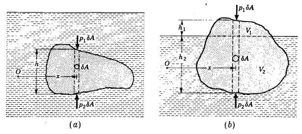
Fig. 2.34. Vertical force components on element of body.
