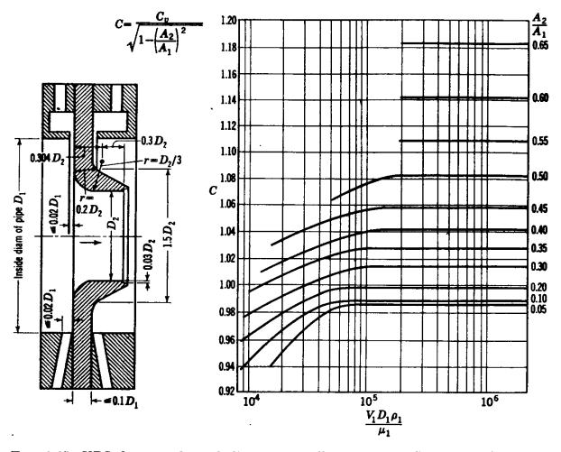
Fig. 9.26. VDI flow nozzle and discharge coefficients. (NACA Tech. Mem. 952, Reference 11.)
