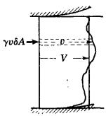
Fig. 3.11. Velocity distribution and average velocity.
