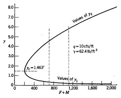
Fig. 11.5. F + M curve for hydraulic jump.
