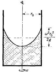
Fig. 2.19. Rotation of circular cylinder about its axis.
