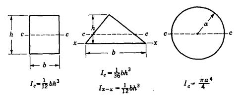
Fig. A.2. Moments of inertia of simple areas about centroidal axes.
