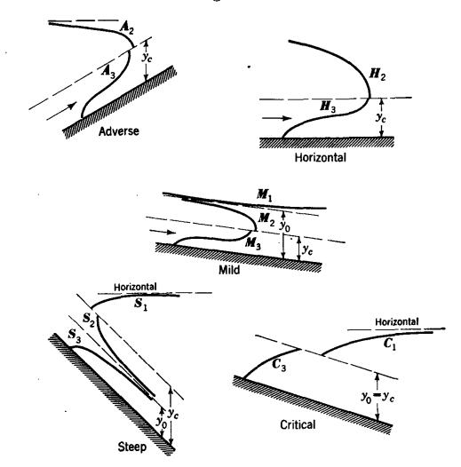
Fig. 11.11. The various typical liquid-surface profiles.
