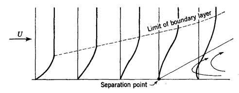
Fig. 5.20. Effect of adverse pressure gradient on boundary layer. Separation.
