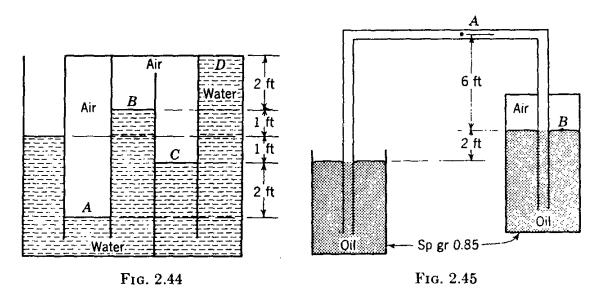
**2.3.** The tube in Fig. 2.45 is filled with oil. Determine the pressure at A and B in feet of water.
