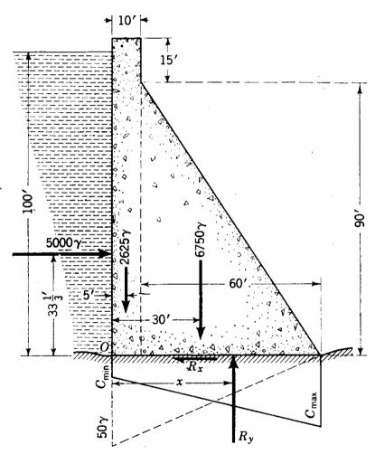
Fig. 2.25. Concrete gravity dam.
