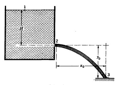
Fig. 9.19. Orifice in a reservoir.
