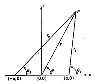
Fig. 7.14. Auxiliary coordinate systems used for Rankine body.
