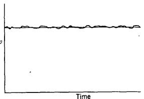
Fig. 3.1. Velocity at a point in steady turbulent flow.
