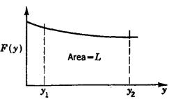
Fig. 11.10. Numerical integration of gradually varied flow equation.
