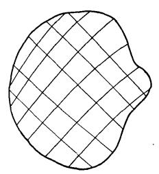
Fig. 3.3b. Decomposition of large volume into elements.
