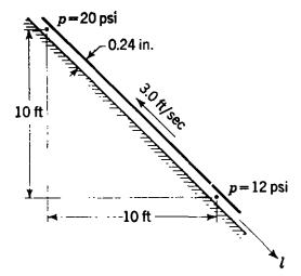
Fig. 5.2. Flow between inclined flat plates.
