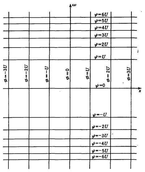
Fig. 7.17. Streamlines and equipotential lines for uniform flow in negative x-direction.
