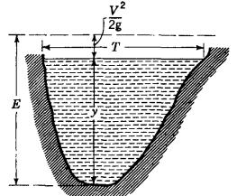
Fig. 11.8. Specific energy for a non-rectangular section.
