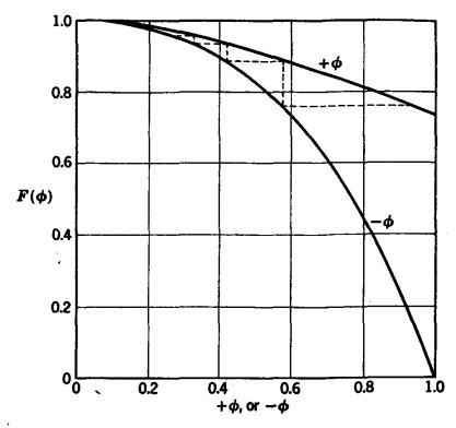
Fig. 10.15. Graphical solution of  $F(\phi) = (1 + \phi)e^{-\phi}$ .
