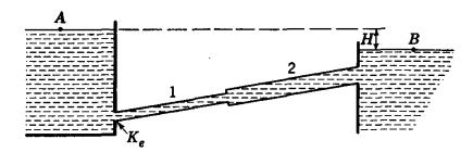
Fig. 10.6. Pipes connected in series.
