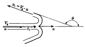
Fig. 8.12. Flow through bucket.
