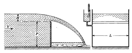
Fig. 9.30. Sharp-crested rectangular weir.
