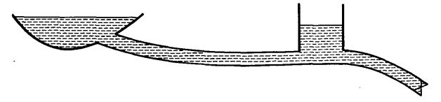
Fig. 10.18, Surge tank on a long pipeline.
