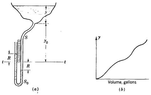
Fig. 2.10. Manometer used for measuring volume in tank.
