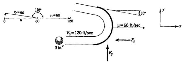
Fig. 3.30. Vector diagram for jet on moving vane.
