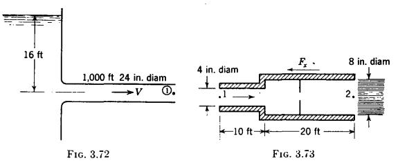
**3.140.** Water fills the piping system of Fig. 3.73. At one instant  $p_1 = 5$  psi,  $p_2 = 0$ ,  $V_1 = 10$  ft/sec, and the flow rate is increasing by 5000 gpm per minute. Find the force  $F_x$  required to hold the piping system stationary.
