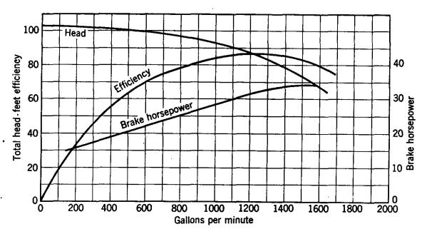
Fig. 8.27. Characteristic curves for typical centrifugal pump. 10-in. impeller, 1750 rpm. (Ingersoll-Rand Co.)
