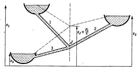
Fig. 10.8. Three interconnected reservoirs.
