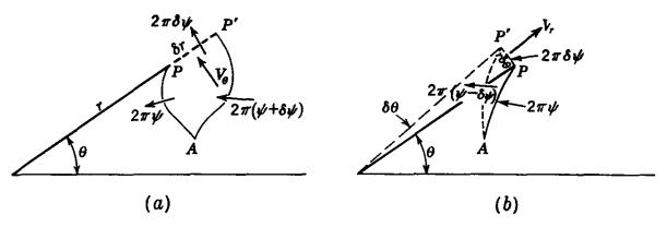
Fig. 7.10. Displacement of P to show the relation between velocity components and Stokes' stream function.
