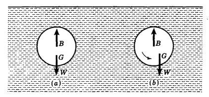
Fig. 2.38. Rotationally stable submerged body.
