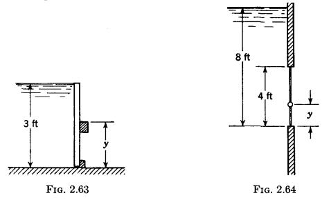
**2.83.** Determine the hinge location y of the rectangular gate of Fig. 2.64 so that it will open when the liquid surface is as shown.
