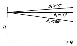
Fig. 8.28. Theoretical head-discharge curves.
