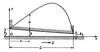
Fig. 5.38. Sliding bearing.
