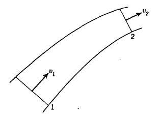
Fig. 3.4. Steady flow through a stream tube.
