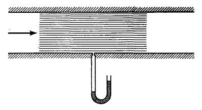
Fig. 9.1. Piezometer opening for measurement of static pressure.
