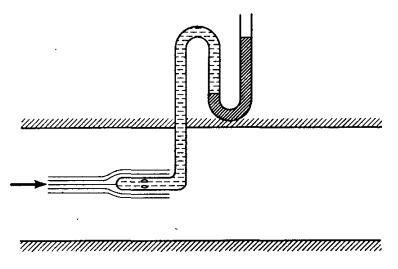
Fig. 9.2. Static tube.
