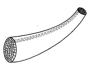
Fig. 3.5. Collection of stream tubes between fixed boundaries.
