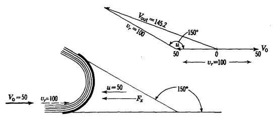
Fig. 3.32. Vector diagram for vane doing work on a jet.
