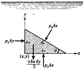
Fig. 2.1. Free-body diagram of wedge-shaped particle.
