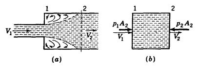
Fig. 3.33. Sudden expansion in a pipe.
