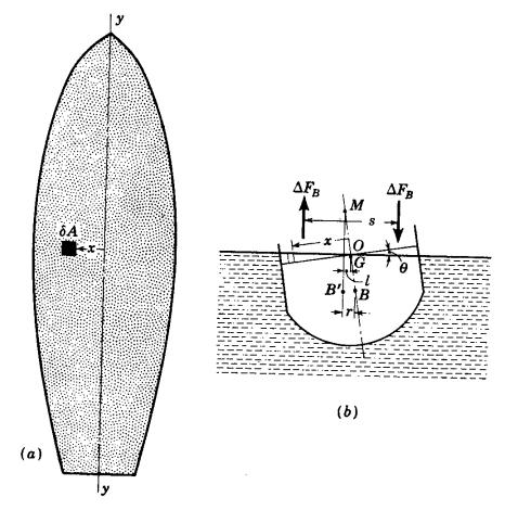
Fig. 2.40. Stability relations in body of variable cross section.
