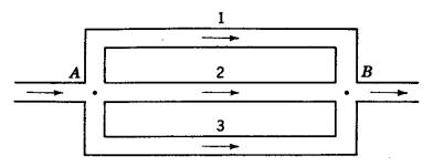
Fig. 10.7. Parallel-pipe system.
