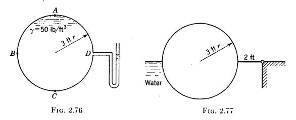
2.110. The cylinder gate of Fig. 2.77 is made up from a circular cylinder and a plate, hinged at the dam. The gate position is controlled by pumping water into or out of the cylinder. The center of gravity of the empty gate is on the line of symmetry 4 ft from the hinge. It is in equilibrium when empty in the position
