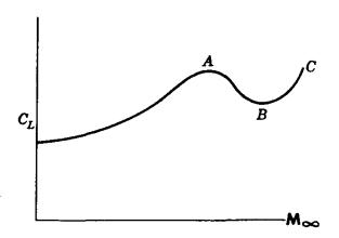
Fig. 6.8. Variation of  $C_L$  through the transonic range.
