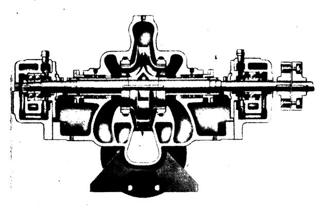
Fig. 8.20. Cross section of a single-stage double-suction centrifugal pump. (Ingersoll-Rand Co.)
