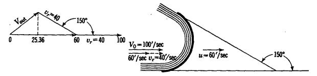
Fig. 3.31. Vector diagram for moving vane.
