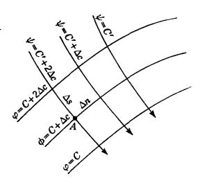
Fig. 7.13. Elements of a flow net.
