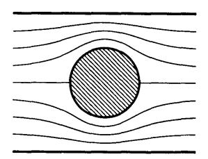
Fig. 3.2. Streamlines for steady flow around a cylinder between parallel walls.
