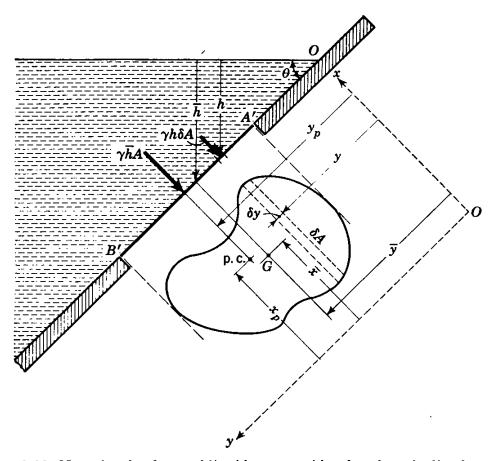
Fig. 2.22. Notation for force of liquid on one side of a plane inclined area.
