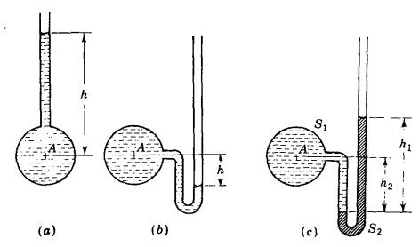
Fig. 2.8. Examples of simple manometers.
