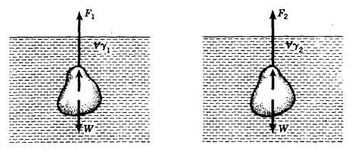
Fig. 2.35. Free-body diagram for body suspended in a fluid.
