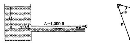
Fig. 3.36. Acceleration of liquid in a Fig. 3.37. Notation for moment of a pipe.
