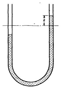
Fig. 10.13. Oscillation of liquid in a U-tube.
