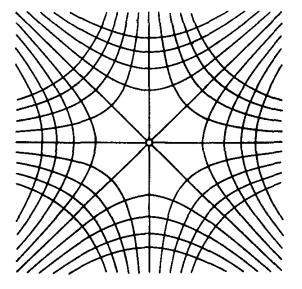
Fig. 7.24. Flow net for flow around 90° bend.
