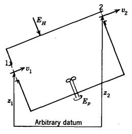
Fig. 3.16. Control volume for steady flow.
