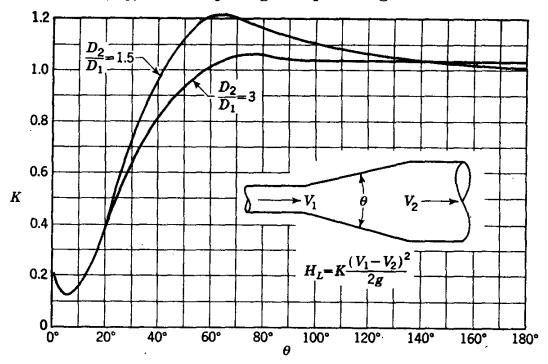
Fig. 5.36. Loss coefficients for gradual conical expansions.
