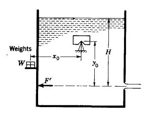
Fig. 9.20. Momentum method for determination of  $C_v$  and  $C_c$ .
