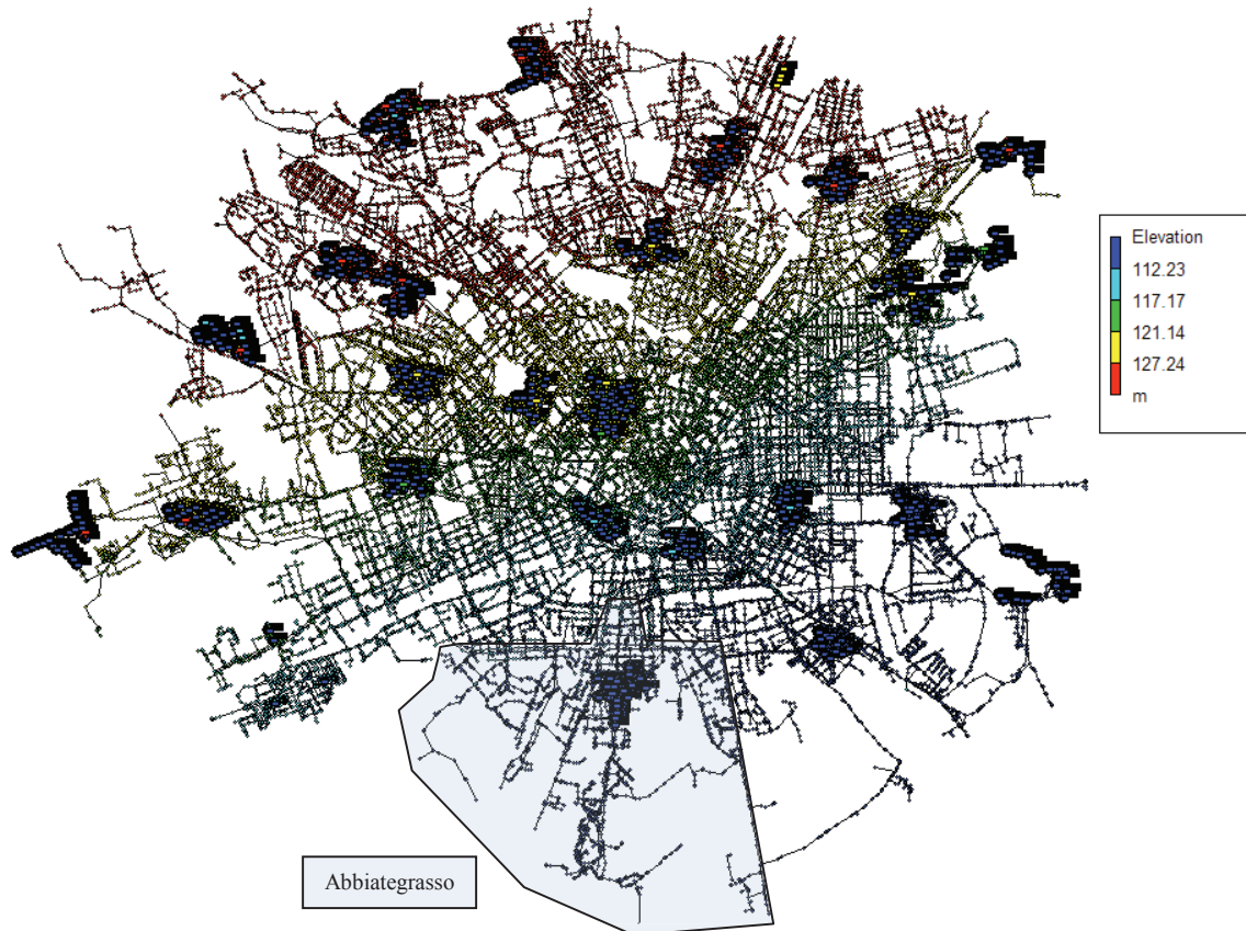
Figure 2. Milano WDN model. Elevations of the elements of the model. Gradient from North to South.
