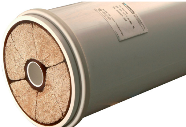
(a) Ultrafiltration membrane cartridge containing more than 15 000 fibres with total surface area about 80 m 2 , treatment capacity 6–8 m 3 /mh. Inset cross section of hollow fibre membrane, internal dia. 0.8 mm. (Manufacturer: Koch Membrane Systems Inc., Wilmington, MA, USA).
