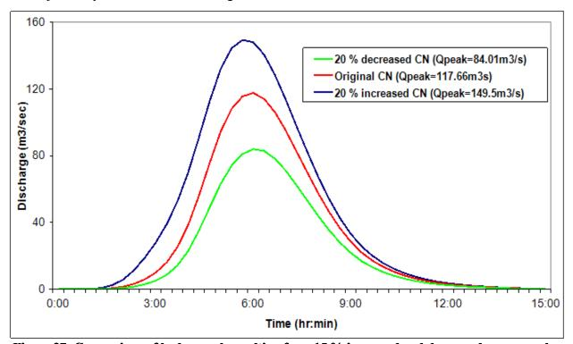
Figure 27: Comparison of hydrograph resulting from 15 % increased and decreased curve number A 15% decrease of the initial abstraction of the study subbasin leads to a decrease of the peak discharge of 28.6%. The 15% increase results in an increase in peak discharge of 18.0%. Therefore, it can be expected that the deviation of the resulting peak discharges from the actual peak discharges is in the range of  $\pm 30$  %.
