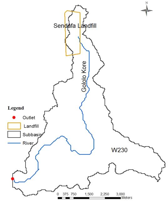
Figure 18: Catchment in the Study Area Delineated using HEC-GeoHMS
