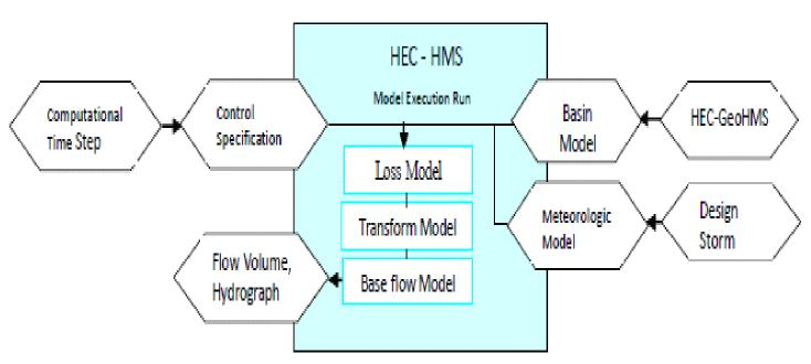
Figure 16: HEC - HMS Software Components
