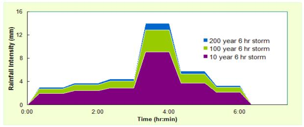
**Figure 33: Six hours design storm hyetographs used for rainfall - runoff modeling** The model predicted flood hydrographs for the study watershed outlet for return periods of 10, 100 and 200 years. The hydrographs related to the design storms with maximum rainfall intensity at 67 % of the total storm duration are shown in the Figure 34.
