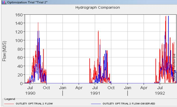
Figure 31: Comparison of Observed and Calibrated Hydrograph
