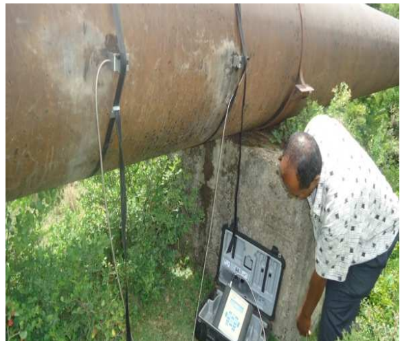
Figure 4.7 Photo of Field flow measurement of 900mm
