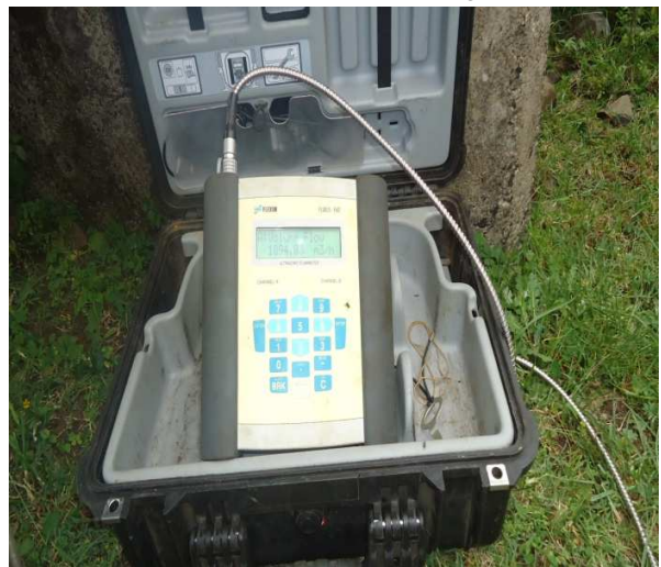
Figure 4.7 Photo of Field flow measurement of 900mm
