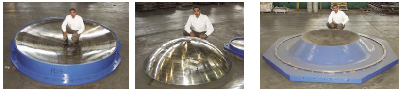
Components of friction pendulum seismic isolator device for a large offshore structure
