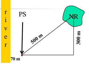
Groundwater is pumped from a confined aquifer. The pumping discharge is 314.2 m<sup>3</sup> day<sup>-1</sup>. The saturated depth of the aquifer is 50 m; the hydraulic conductivity of the aquifer equals 10 m day<sup>-1</sup> and the storage coefficient of the aquifer is 0.0001. A river is located at a distance of 70 m of the pumping station (PS), and the midpoint of a nature reserve (NR) is located at a distance of 500 m from the pumping well.
