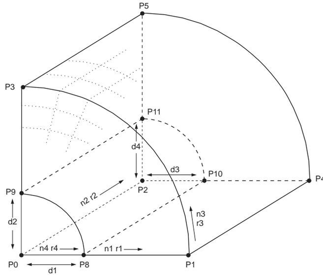
Figure 1.20 Cylinder shell mesh — cshell
