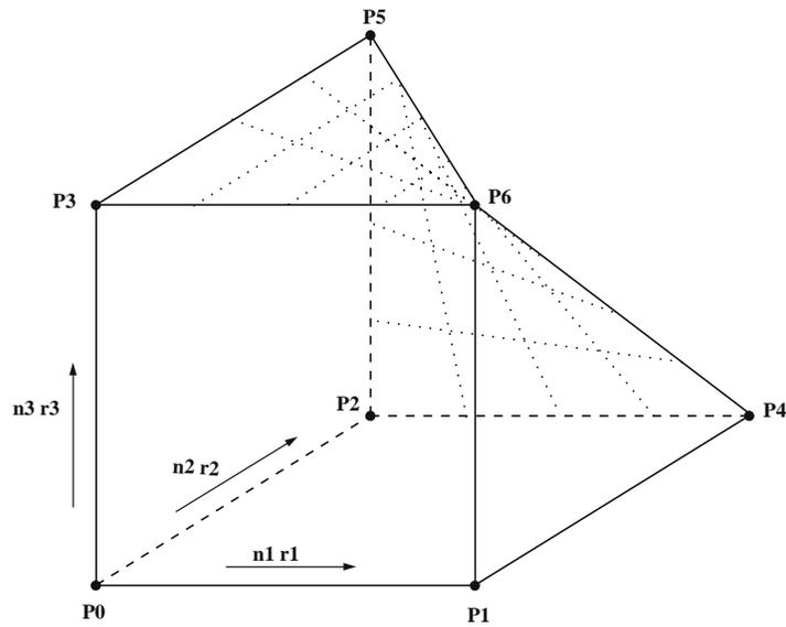
Figure 1.11 Degenerate brick mesh — dbrick
