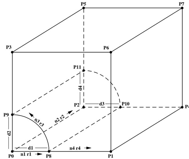
Figure 1.19 Radially graded mesh around cylindrical-shaped tunnel — radcylinder
