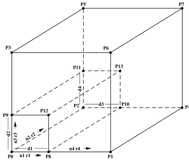
Figure 1.18 Radially graded mesh around parallelepiped-shaped tunnel — radtunnel
