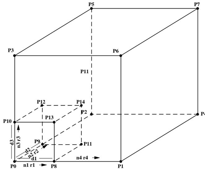
Figure 1.17 Radially graded mesh around brick — radbrick
