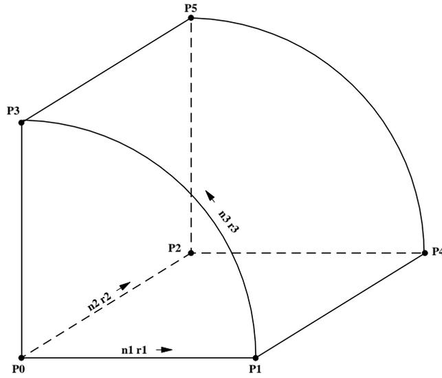
Figure 1.16 Cylindrical mesh — cylinder
