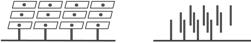
Figure 9.7.14 Impedance structures of mushrooms and straight pins.
