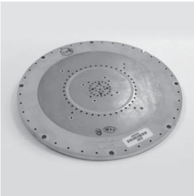
Figure 9.7.7 Dual frequency concentric patch antenna board of Legant antenna.
