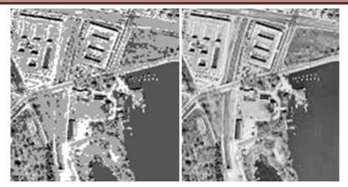
Figure 5-10 Radiometric Resolution
