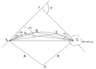
Figure 3-8 Setting out by two theodolite method
