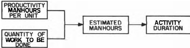
FIGURE 5.10 Process for Determining Activity Duration
