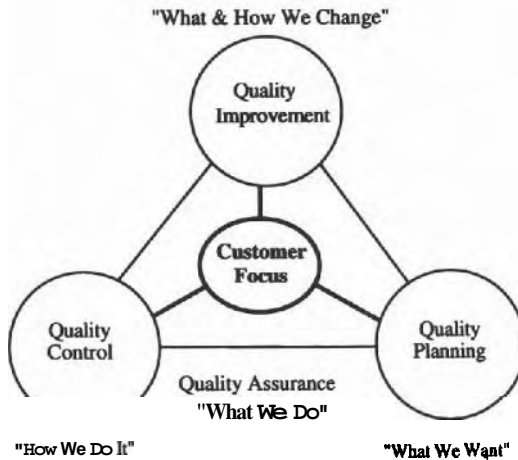
FIGURE 22.2 Scope of Quality Management with a Customer Focus
