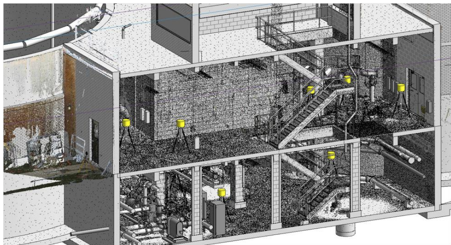
FIGURE 21.1 Creating as-built drawings. The black-and-white scan data in the background is represented as a granular series of points.
