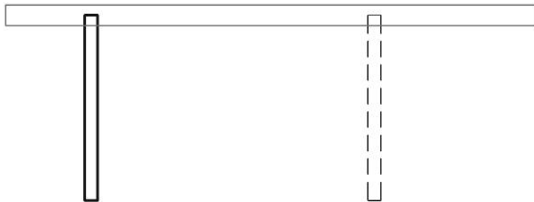
FIGURE 12.24 Walls with disallowed joins will overlap.
