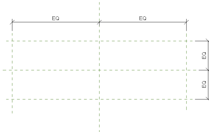
FIGURE 14.19 Set equality constraints on reference planes first.
