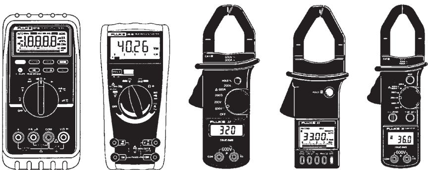
Figure 6.8 True rms digital multimeters. (Reproduced with permission of Fluke Corp.©)
