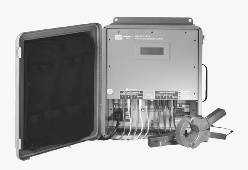
Figure 6.25 Permanent power quality monitor. (Courtesy of Dranetz-BMI.)
