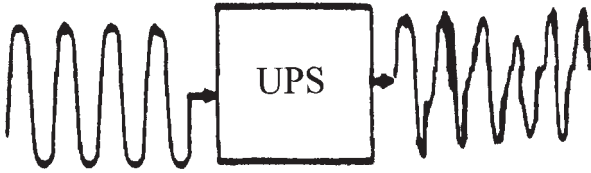
Figure 7.2 UPS distorted power.
