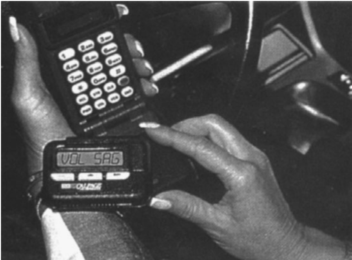
Figure 6.16 Power quality pager. (Courtesy of Dranetz-BMI.)
