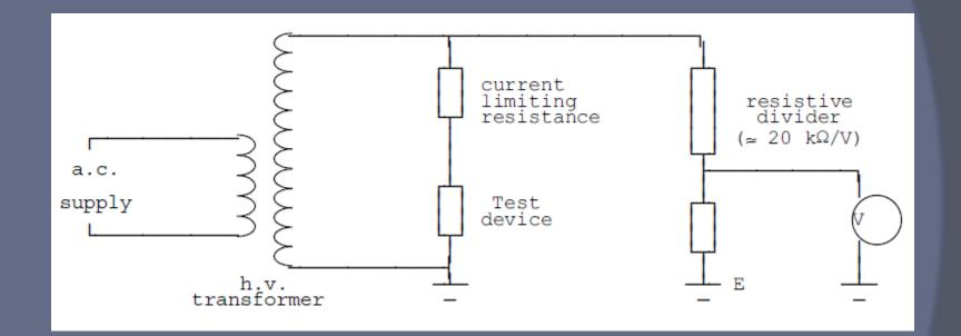
In this method, a high resistance potential divider is connected across the highvoltage winding, and a definite fraction of the total voltage is measured by means of a low voltage voltmeter.
