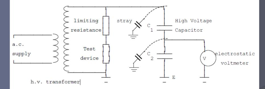
For AC, instead of using a resistive potential divider, we could use a capacitive potential divider. In this two capacitances C1 and C2 are used in series, the electrostatic voltmeter being connected across the lower capacitor.
