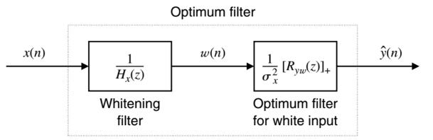
• Where, the whitening filter has to satisfy  $R_x(z) = \sigma_x^2 H_x(z) H_x^* \left(\frac{1}{z^*}\right)$  Spectral factorization • Then y(n) is estimated from the white noise with  $H'_{c}(z) = \frac{1}{\sigma_{x}^{2}} [R_{yw}(z)]_{+}$
