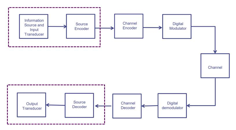
Functional block diagram of a typical digital communication system
