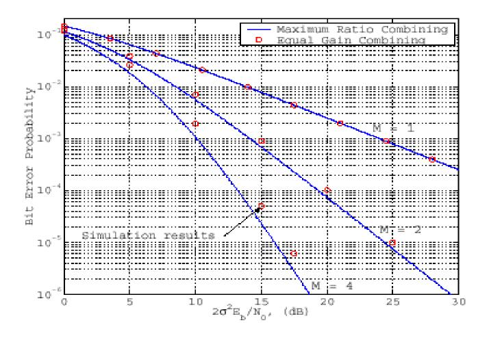
Average bit error probability of coherent BPSK with EGC over Rayleigh fading channels
