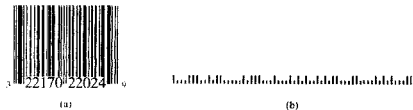
Figure 12.1 Two forms of linear bar codes: (a) width-modulated, exemplified here by the Universal Product Code; and (b) height-modulated, exemplified here by Postnet, used by the U.S. Postal Service.
