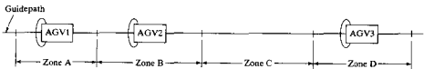
Figure 10.5 Zone control to implement blocking system. Zones A, B, and D are blocked. Zone C is free. Vehicle 2 is blocked from entering Zone A by Vehicle 1. Vehicle 3 is free to enter Zone C.
