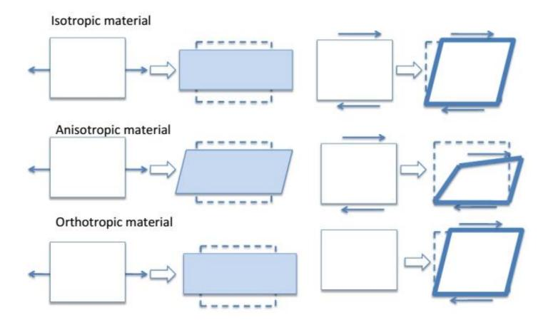
When stressed along the principal directions an orthotropic materials deforms as an isotropic one
