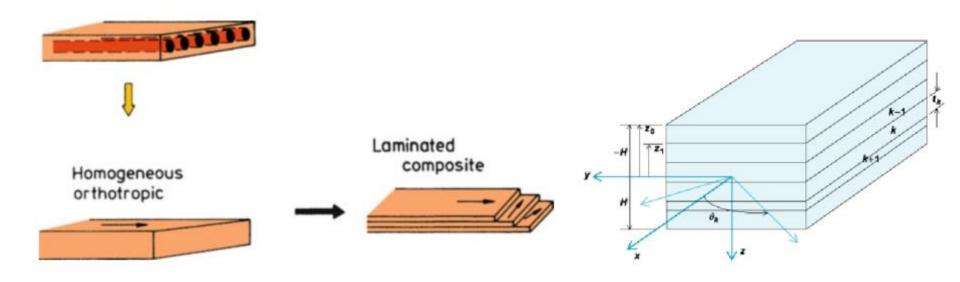
A laminate is made by stacking laminae with different fiber orientations tailored to fulfill specific mechanical requirements in specific directions. Usually, the laminae have the same thickness, same matrix/fibers, and the same fiber content.
