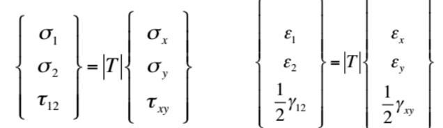
Where  $\gamma_{xy}$  is the engineering strain, and  $\frac{1}{2} \gamma_{xy}$  is the tensorial strain
