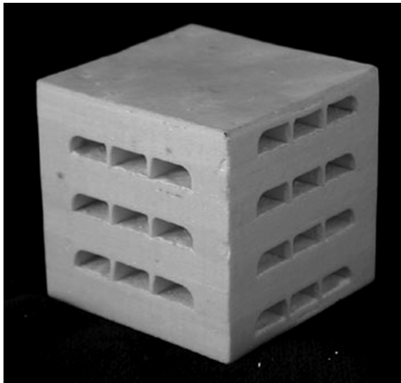
FIGURE 3.8 Small (~5 cm × 5 cm × 5 cm) ceramic heat exchanger model illustrating a plate–fin-layered cross-flow design. (Sample fabricated in the 1970s by GTE Sylvania.) (Photo by D. W. Richerson.)
