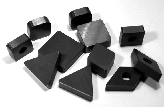
FIGURE 3.29 Variety of silicon nitride ceramic cutting tool inserts. Typical size is 1–2 cm. (Photo by D. W. Richerson.)
