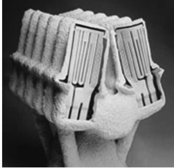
FIGURE 3.2 Cutaway view of a ceramic investment casting mold for fabrication of gas turbine engine rotor blades showing the ceramic cores for producing the complex internal cooling passages in the cast metal blades. Fabricated by Howmet Research Corporation, Whitehall, Michigan. The cutaway section is ~12 cm tall by 5 cm wide. (Reprinted from Richerson, D. W., The Magic of Ceramics , American Ceramic Society, Westerville, OH, 2000, p. 224. With permission of the American Ceramic Society, www.ceramics.org .)
