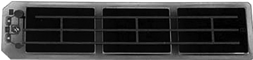
FIGURE 3.38 Piezoelectric module for a K2 “smart ski” that consists of three ceramic wafers imbedded in plastic and connected to high-resistance electrical wiring. When the ski begins to vibrate as the skier goes faster and faster, some of the vibrations are converted by the piezoelectric ceramic into electricity that is then converted into heat by the high electric resistance wiring. The module manufactured by Active Control eXperts, Cambridge, Massachusetts, is 16.8 cm long. (Photo by D. W. Richerson.)
