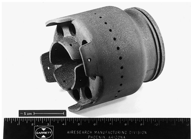
FIGURE 13.36 Annular combustor for a gas turbine engine fabricated by drain casting using nonabsorbing pins and mandrels inserted into the mold (fabricated by Norton Company [currently Saint-Gobain/Norton Advanced Ceramics]). (Courtesy of Garrett Turbine Engine Company [currently Honeywell Engines, Systems & Services, Phoenix, AZ].)
