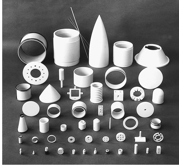
FIGURE 13.21 Ceramic parts formed by uniaxial and isostatic pressing, some with green machining. (Courtesy of Western Gold and Platinum Company, Belmont, CA, Subsidiary of GTE Sylvania, Inc.)
