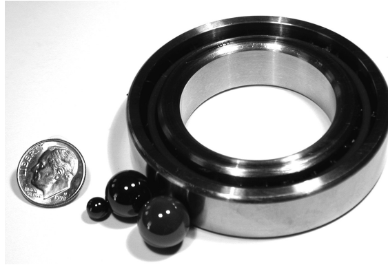
FIGURE 3.25 Silicon nitride ceramic bearing balls (fabricated by Saint-Gobain Advanced Ceramics, East Granby, CT) and an assembled hybrid bearing with silicon nitride balls in a metal race. The size is compared to a US dime, which is about 1.3 cm across. (Photo by D. W. Richerson.)
