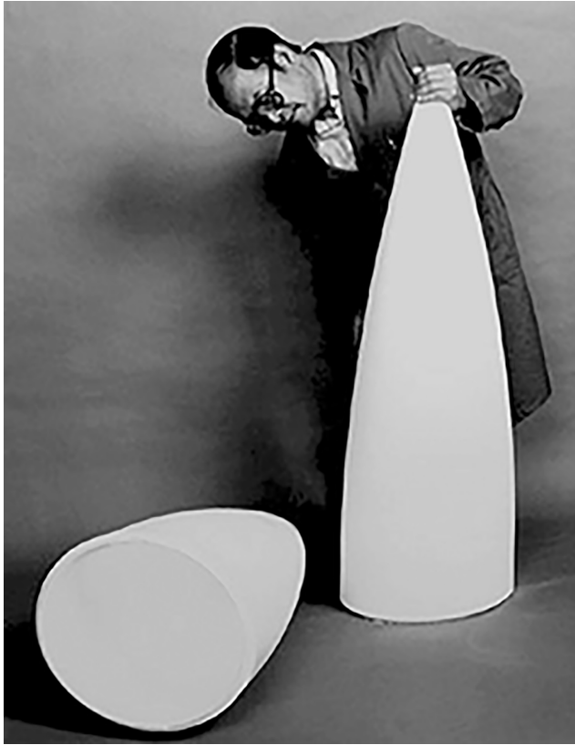
FIGURE 3.60 Ceramic radomes to perform as electromagnetic windows to allow electromagnetic waves of specific frequencies and wavelengths to pass through to the electronic equipment inside. (Reprinted from Richerson, D. W., The Magic of Ceramics , American Ceramic Society, Westerville, OH, 2000, p. 69. With permission of the American Ceramic Society, www.ceramics.org ; courtesy of Ceradyne, Costa Mesa, CA.)
