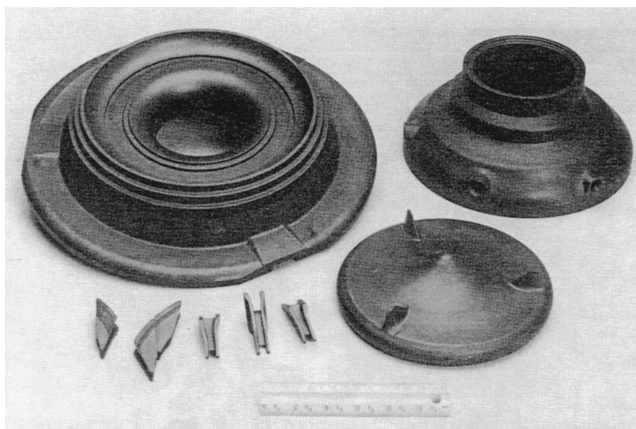
FIGURE 14.12 SiC gas turbine components fabricated using \alpha -SiC powder plus B and C sintering aids. (Courtesy of Carborundum Company for parts fabricated for Garrett Auxiliary Power Division of Allied-Signal Aerospace during the 1980s under sponsorship of the US Department of Energy and Administration of NASA-Lewis Research Center.)
