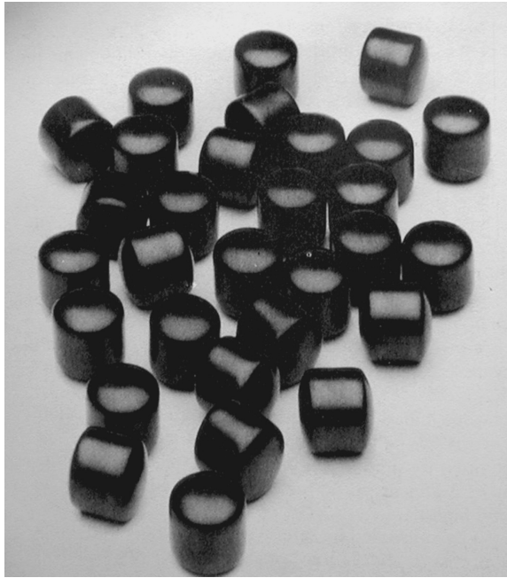
FIGURE 12.12 \text{Si}_3\text{N}_4 grinding media showing one of the common configurations. Spheres are also commonly used. (Courtesy of KemaNord, Sweden.)
