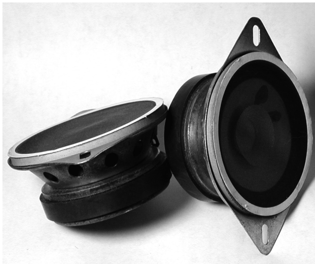
FIGURE 3.43 Ceramic magnets (8.5 cm diameter) built into the backside of a loudspeaker. (Photo by D. W. Richerson.)
