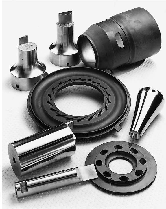
FIGURE 15.3 Examples of shapes fabricated by ultrasonic machining. (Courtesy of Bullen Ultrasonics, Inc., Eaton, OH.)
