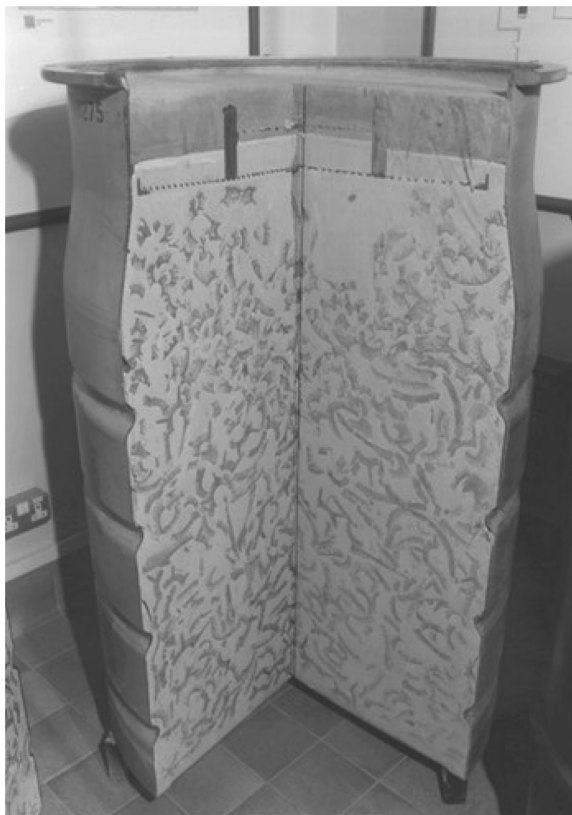
FIGURE 21.17 Cut away of a cement-encapsulated ILW in a 500 L steel drum. (Courtesy of National Nuclear Laboratory, Cumbria.)
