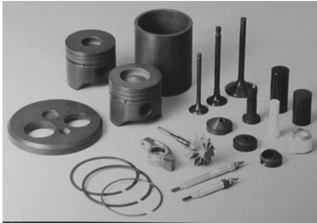
FIGURE 3.14 Experimental ceramic parts evaluated for automotive engines plus a few production parts. (Courtesy of Kyocera Corporation, Kyoto, Japan; reprinted from Richerson, D. W., The Magic of Ceramics , American Ceramic Society, Westerville, OH, 2000. With permission of the American Ceramic Society, www.ceramics.org.)
