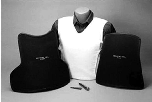
FIGURE 3.61 Boron carbide personnel armor with the projectiles that it can defeat. (Reprinted from Richerson, D. W., The Magic of Ceramics , American Ceramic Society, Westerville, OH, 2000, p. 259. With permission of the American Ceramic Society, www.ceramics.org ; courtesy of Ceradyne, Costa Mesa, CA.)
