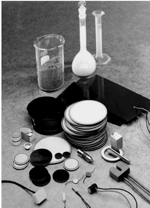
FIGURE 3.54 Piezoelectric ceramic parts for medical applications. The powders from which the piezoelectric materials are synthesized are shown at the top. The samples at the lower left and right with the wires connected are for kidney dialysis bubble detectors. The dark samples are coated with a glaze and are built into handheld physical therapy equipment. (Reprinted from Richerson, D. W., The Magic of Ceramics , American Ceramic Society, Westerville, OH, 2000, p. 185. With permission of the American Ceramic Society, www.ceramics.org ; courtesy of Edo Corporation Piezoelectric Products, Salt Lake City, UT.)
