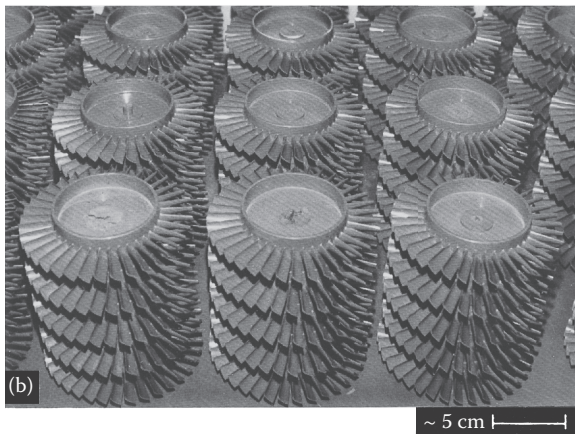
FIGURE 13.68 Complex shapes made by injection molding. (a) Integral stators. (b) Rotor blade rings. (Courtesy of Ford Motor Company, Dearborn, MI.)
