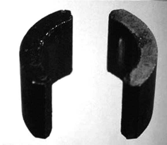
FIGURE 3.42 Ceramic magnets for a windshield wiper motor for an automobile. (Reprinted from Richerson, D. W., The Magic of Ceramics , American Ceramic Society, Westerville, OH, 2000. With permission of the American Ceramic Society, www.ceramics.org .)
