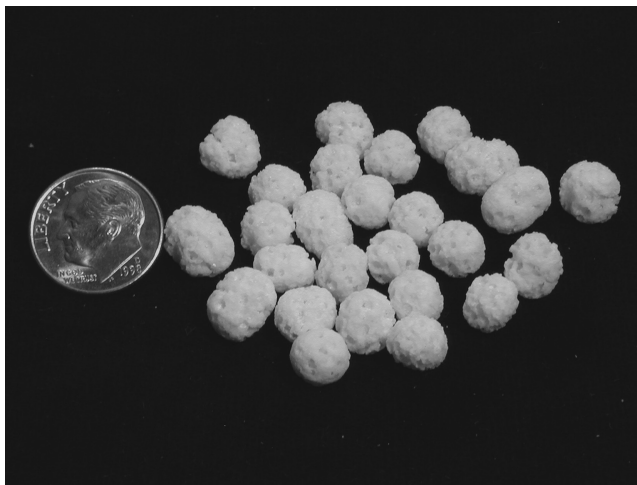
FIGURE 3.10 Porous ceramic beads with high surface area to provide catalytic sites to accelerate chemical reactions in chemical processing. (Samples manufactured by Saint-Gobain Norpro Corporation, Akron, OH.) (Photo by D. W. Richerson.)
