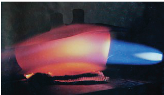
FIGURE 21.20 Silicon nitride gas turbine stator vane surviving a severe thermal shock test that simulated conditions inside the hot section of a gas turbine engine. The test was conducted at Garrett Turbine Engine Company during the late 1970s under a Defense Advanced Research Projects Agency-funded program.
