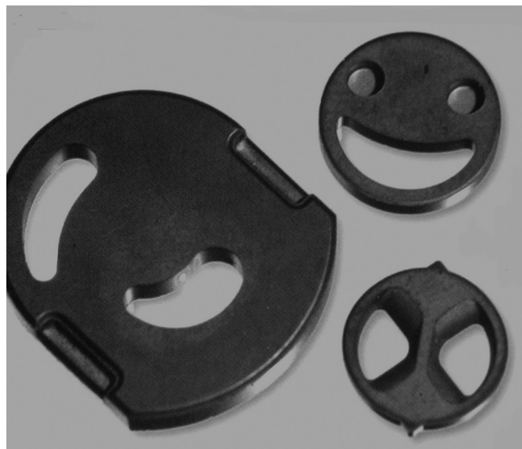
FIGURE 3.19 SiC ceramic pieces for a sink faucet valve and seal, the largest is about 5 cm across. (Photo by D. W. Richerson.)
