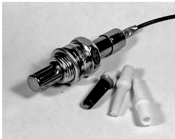
FIGURE 3.39 Oxygen sensor assembly, two as-fabricated doped zirconia solid electrolyte oxygen ion conductor parts, and a finished doped zirconia oxygen ion conductor coated with metal electrodes on the inside and outside and a porous wear-resistant spinel ceramic on the outside. This finished part is 2.8 cm long. (Photo by D. W. Richerson.)
