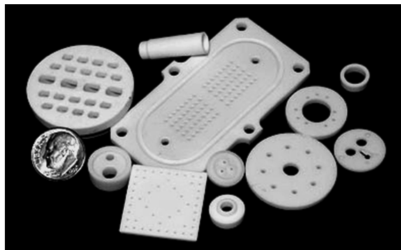
FIGURE 3.33 Variety of small alumina electrical insulators. (Photo by D. W. Richerson.)
