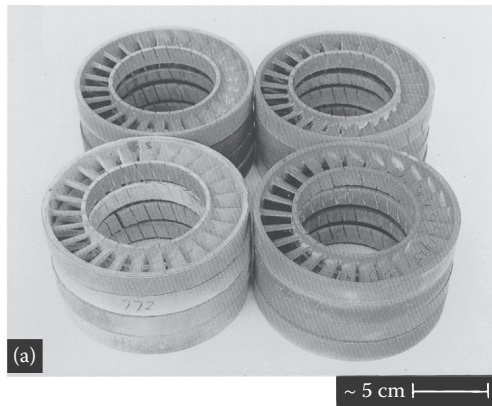
FIGURE 13.67 Prototype sintered silicon nitride turbocharger rotors fabricated by injection molding. (Courtesy of Division of Honeywell Engines, Systems and Services, Airesearch Casting Company, Torrance, CA.)
