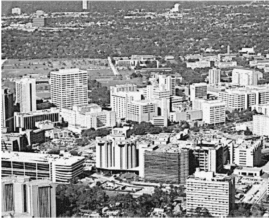
EXPOSURE B STRUCTURES IN THE FOREGROUND ARE LOCATED IN EXPOSURE B. STRUCTURES IN THE CENTER TOP OF THE PHOTOGRAPH ADJACENT TO THE CLEARING TO THE LEFT, WHICH IS GREATER THAN APPROXIMATELY 656 FT (200 M) IN LENGTH, ARE LOCATED IN EXPOSURE C WHEN WIND COMES FROM THE LEFT OVER THE CLEARING. (SEE FIGURE C6-5.)
