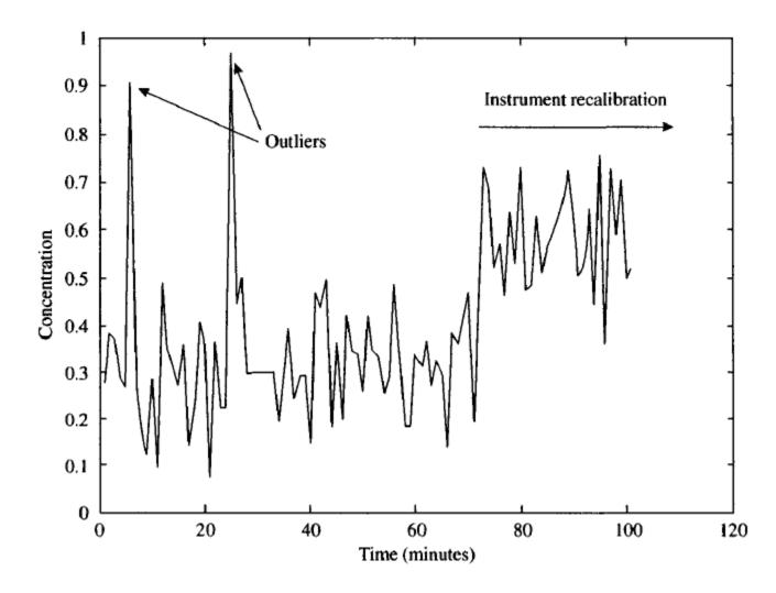
• The first part (in time) of the shows **two big outliers and a slow trend**. These anomalies initiated a recalibration of the corresponding instrument which is seen in the form of a positive jump on the plot
