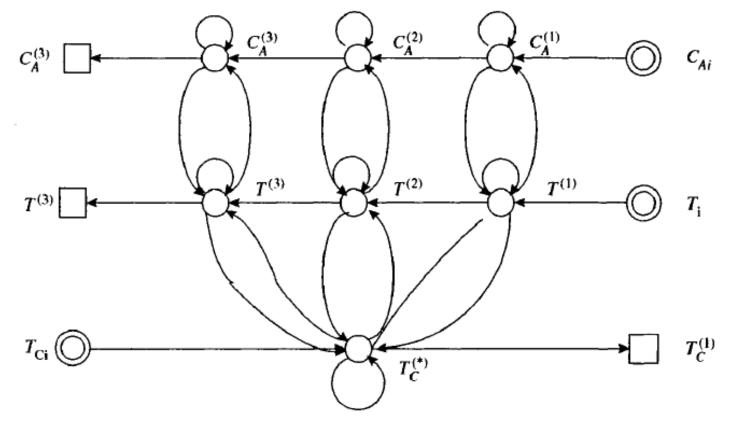
• Simplified structure graph of three jacketted CSTRs by variable removal.
