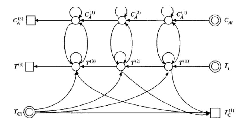
Simplified structure graph of three jacketted CSTRs by variable removal
