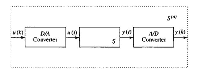
The box labelled S is the original continuous time process system, the box D/A converter converts continuous time signals to discrete time ones and the box A/D converter converts discrete time signals to continuous time ones.  The sampled data discrete time composite system S<sup>d</sup> is in the dashed line box. The discrete time input and output variables (or signals) to the discrete time system S<sup>d</sup> are
