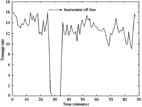
• **Two jumps forming a gross error** are seen in the Figure. The reason for the gross error was a measurement device failure: the corresponding automated sensor went off-line when the first jump was observed and then went back online causing the second jump.
