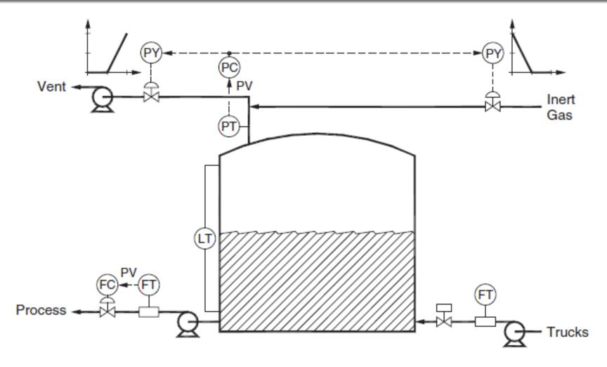
Figure 2.13 Oil storage tank with two feedback controllers
