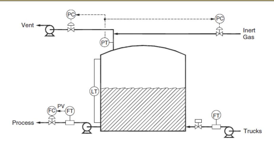
Figure 2.12 Oil storage tank with two feedback controllers
