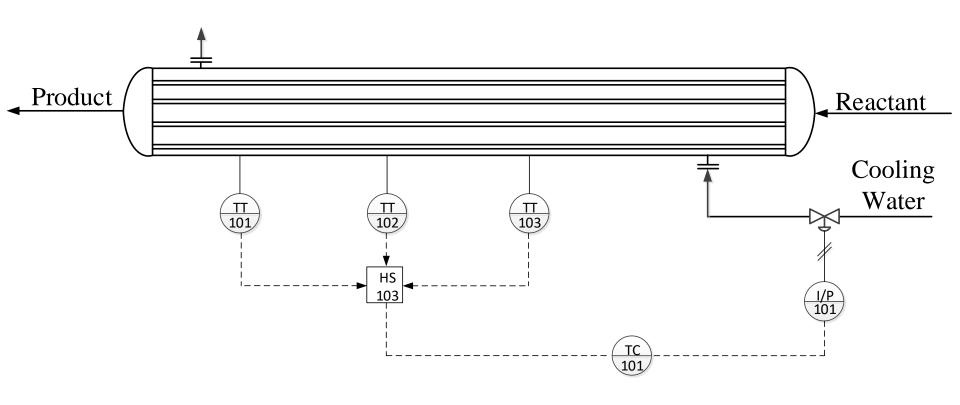
Figure 2.1 A fixed-bed catalytic tubular reactor with an exothermic reaction.
