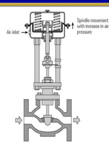
Fail Closed (Air to open), direct acting valve
