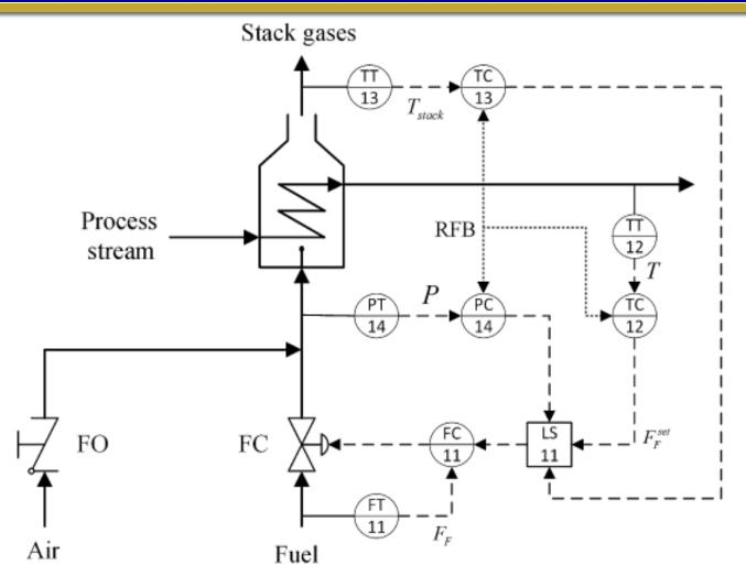
Figure 2.7 Furnace override control
