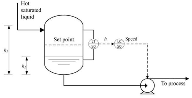
Figure 2.2 Level Control-Feedback
