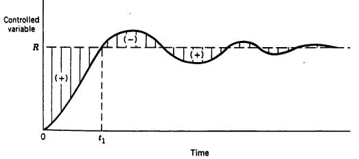
Figure 8.7. Reset windup during a set-point change.
