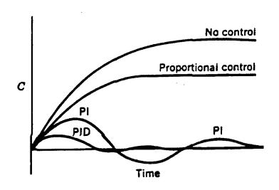
Figure 8.9. Typical process responses with feedback control. No control New steady state is reached P control Offset reduced PI control Offset eliminated Oscillatory response PID control Oscillations reduced No offset
