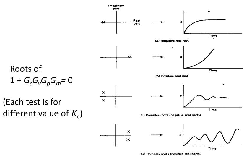
Figure 11.5. Contributions of characteristic equation roots to closed-loop response.
