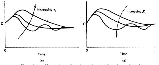
Figure 8.11. PI control: (a) effect of reset time (b) effect of controller gain.
