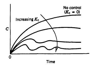
Figure 8.10. Proportional control: effect of controller gain.
