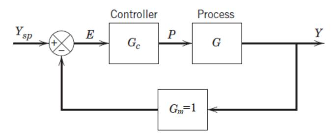
The closed-loop equation for servo problem is given by
