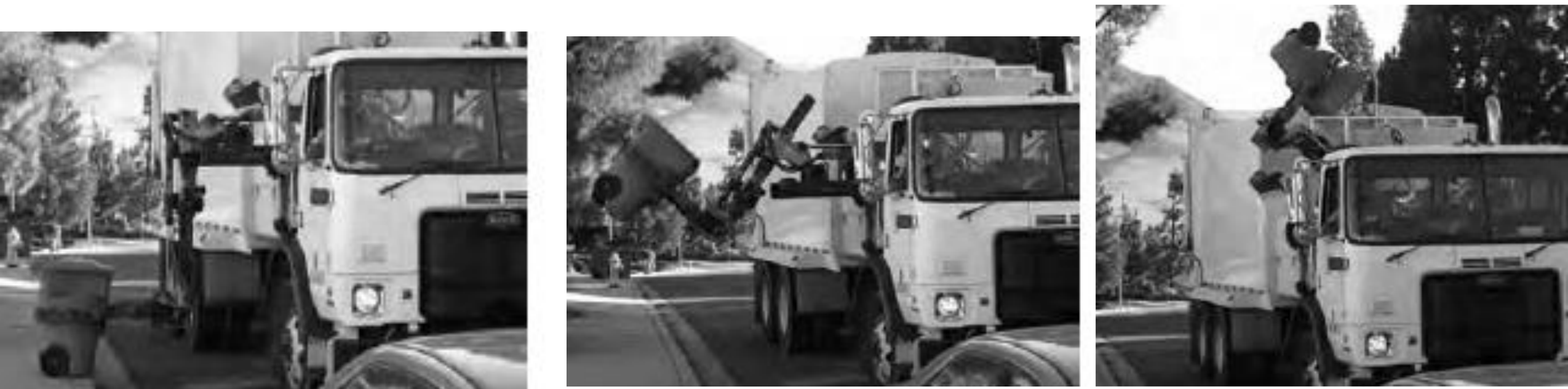
Figure 3-7 Collection with vehicles equipped with “can snatchers.” (Courtesy Peter Cron)
