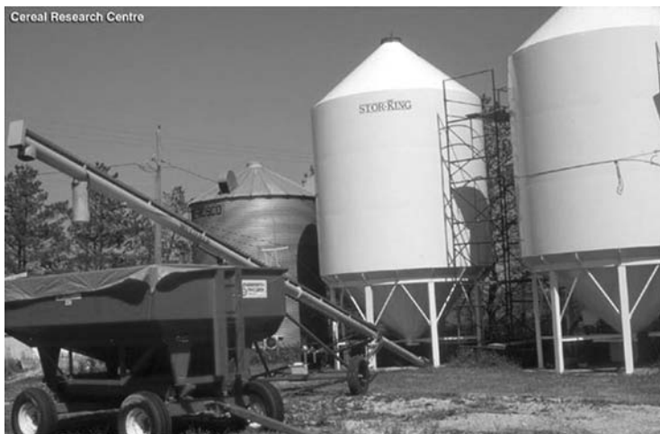
FIGURE 4.43 Hopper-bottom bins. (From CRC. Agriculture and Agri-Food Canada. Winnipeg: Cereal Research Center.)
