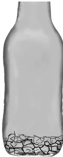
Figure 4.18. Water Hammer Failure in Glass Bottle
