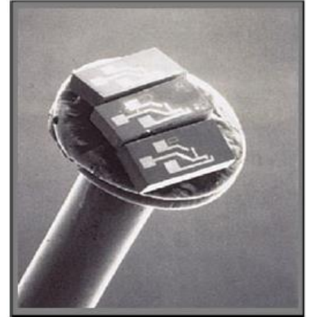
Blood Pressure sensor on the head of a pin
