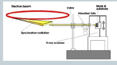
Figure2: Synchrotron Light Source setup
